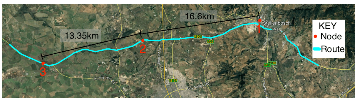
Figure 8.17: Map showing the placement of WSN nodes after the maximum distance finding test. The server node (1) was placed on the Engineering building, while node 2 (2) was placed 16.6 km away, and node 3 was placed 13.35 km away from node 2. The 46 km route which was driven during the on-animal to WSN node test is also shown on the map.
