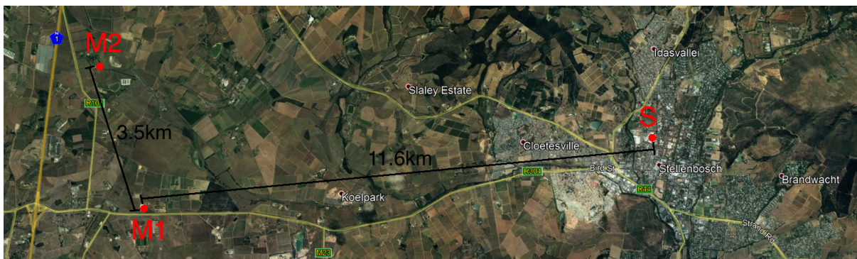
Figure 8.18: Map showing the placement of the WSN nodes for the routing over extended distance tests. The server node (S) was placed on the roof of the Engineering building, and mesh node 1 (M1) was placed 11.6 km away from the server node. Mesh node 2 (M2) was placed 3.5 km from mesh node 1. An on-animal tag sent 50 messages to mesh node 2, which was routed through mesh node 1 to the server node.
