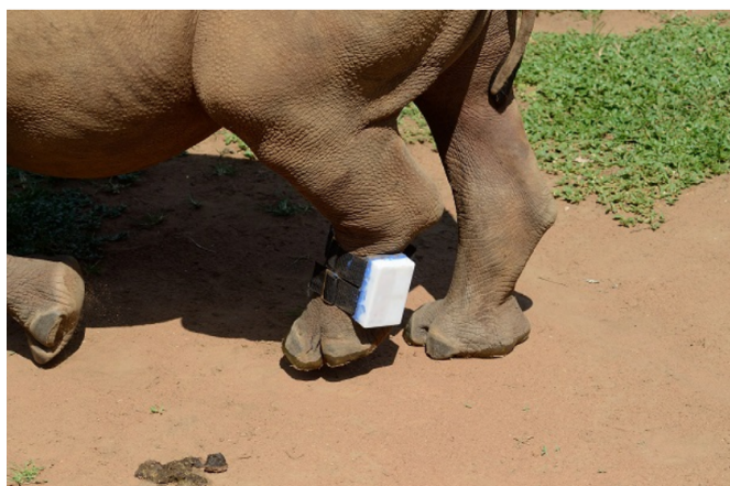
Figure 3.1: Animal tag mounted on the ankle of a rhino. Reproduced from [13].
