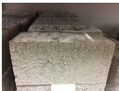
Blocks in curing room
