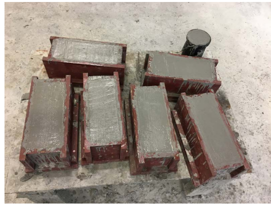
Figure 3.11: AACB Curing in Wooden Mould
