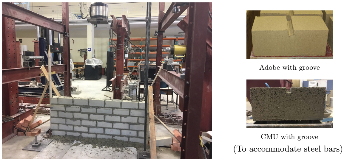
Figure 5.10: Typical Construction of a Wall Specimen
