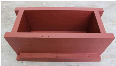
Figure 3.10: AACB Wooden Mould
