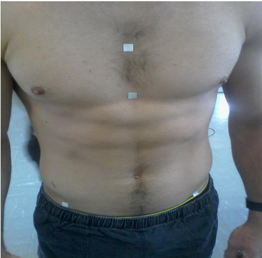
Figure 3.4: Reflective marker placement on participant (photograph by K. Schütte)
