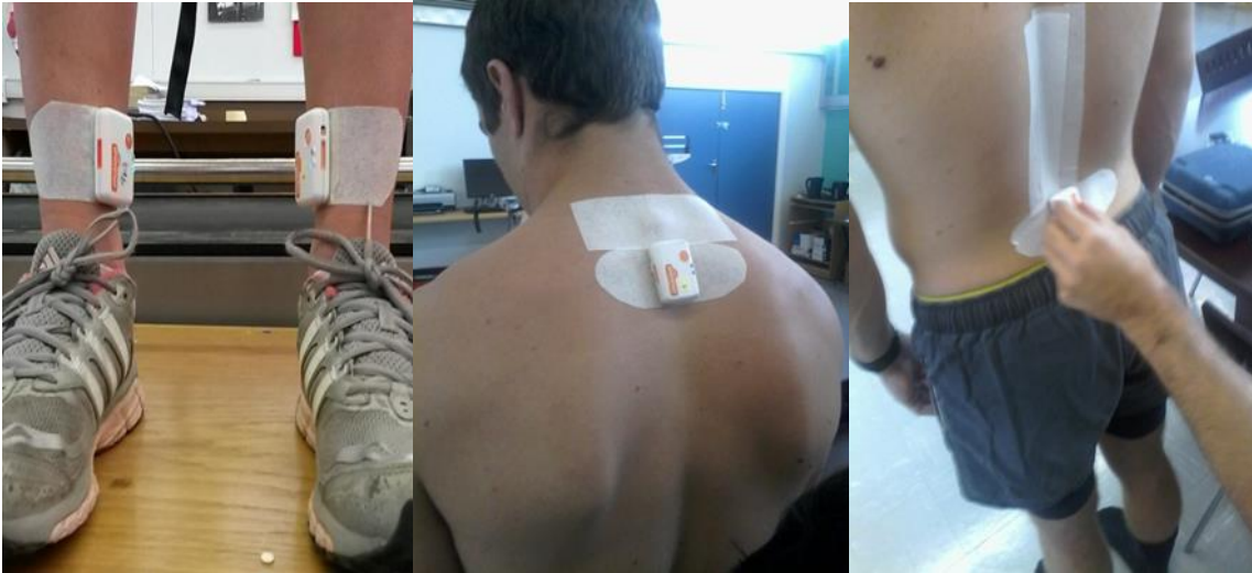
Figure 3.5: Pictures of accelerometer placement (photograph by R. Venter).
