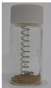
Fig. 3.1 Hygrostat system for accelerated stability tests (40 °C/75% RH) with stainless steel spring, glass conical insert with saturated NaCl solution and clear 24 ml vial (in actual experiments amber vials were used) sealed with PTFE caps
