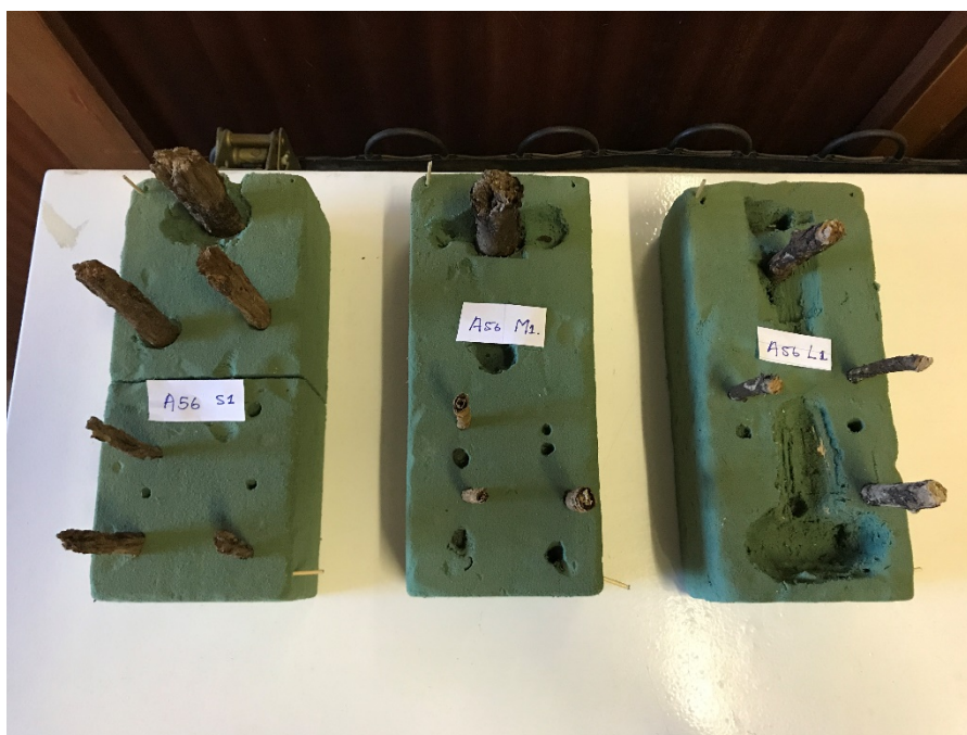
Figure 3.11: Stacking of root samples on phenolic foam blocks before being scanned in the CT-scanner.
