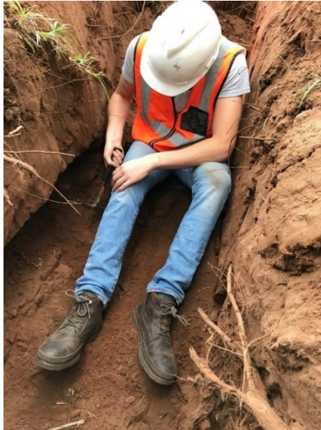
Figure 3.6: Roots being carefully exposed by hand using several tools (geological hammer, paint brushes, tooth brushes and hand shovels) following the excavation of the trench.
