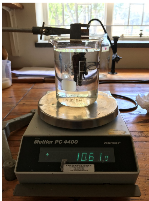
Figure 3.10: Application of the displacement method for determining sample volume
