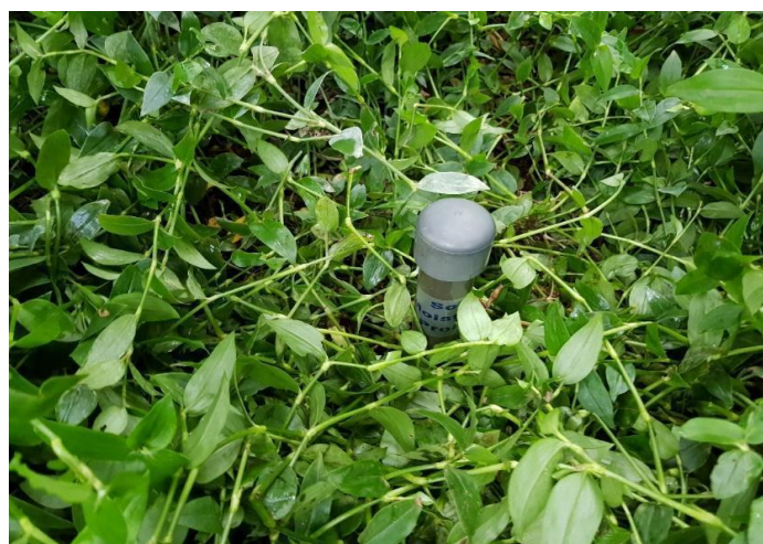
Fig. 3. DFM® continuous logging probe placed in the Tradescantia mulch (TO treatment).
