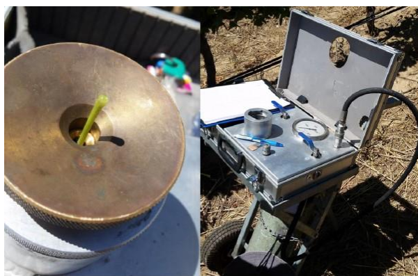
Figure 3.2 Customised pressure chamber used to measure Stem Water Potential.
