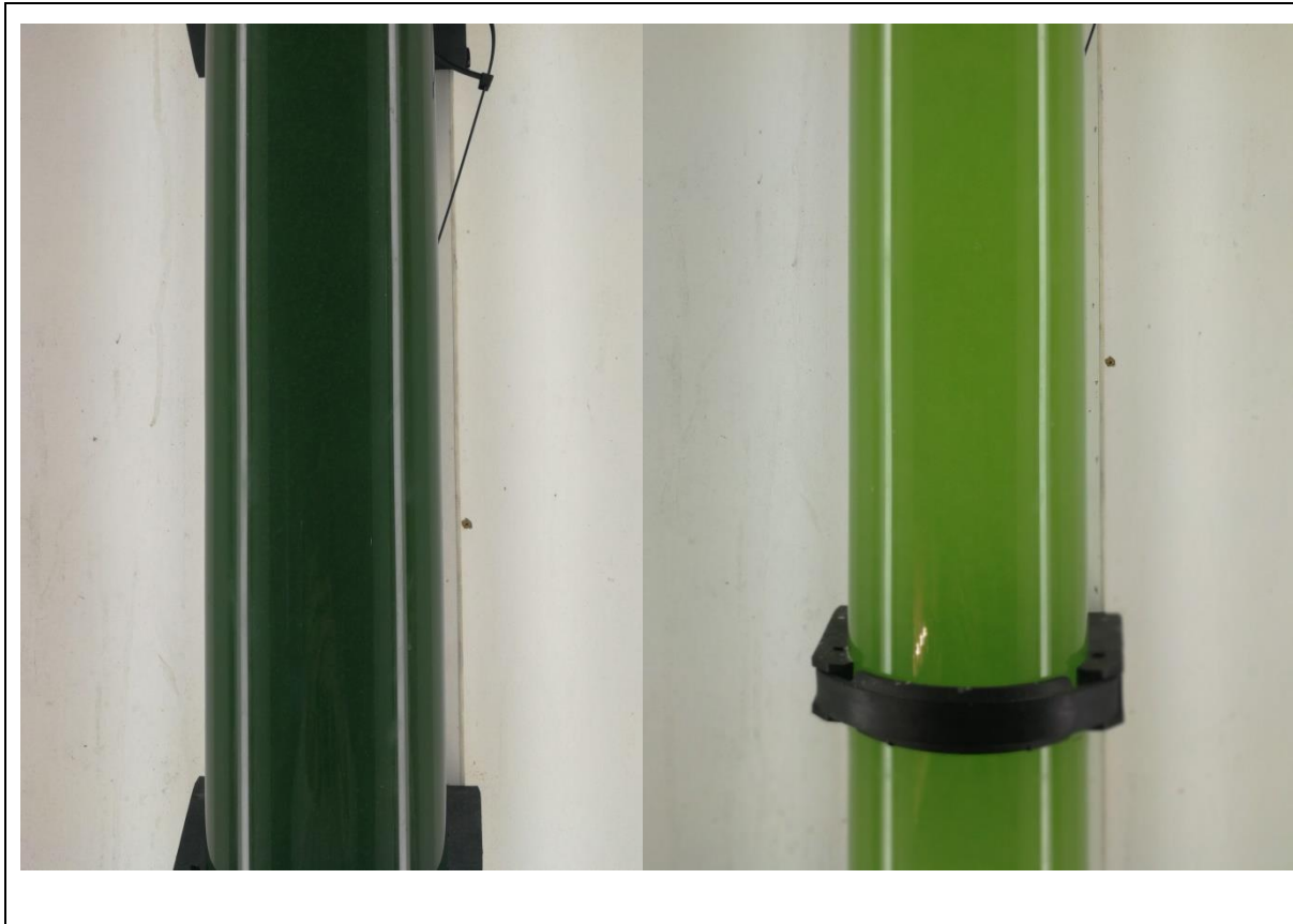
Figure 25: Pictures of Synechococcus PCC 7002 grown in an airlift reactor after 10 days in optimised AD effluent (left) and synthetic media (right) (23 °C; 180 \mu\text{E}\cdot\text{m}^{-2}\cdot\text{s}^{-1} , pH = 6.8)
