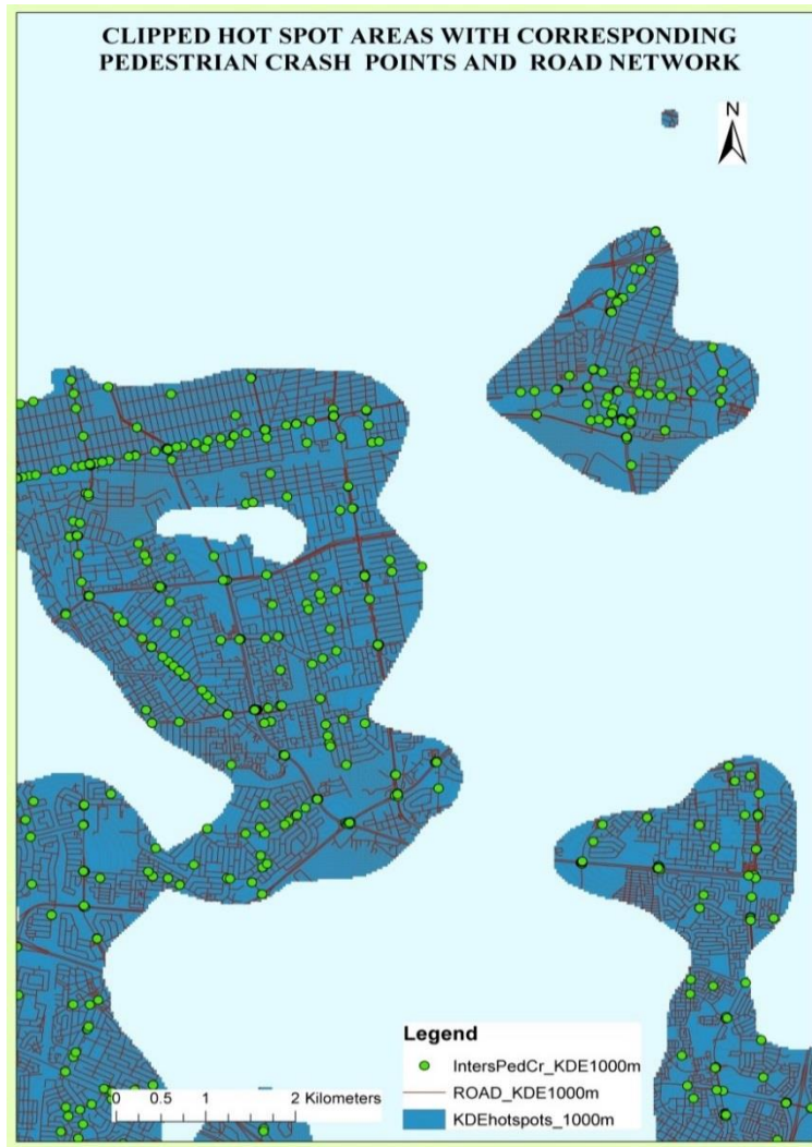
Figure 4-71: An example of clipped KDE hot spots with casualty points and the road network
