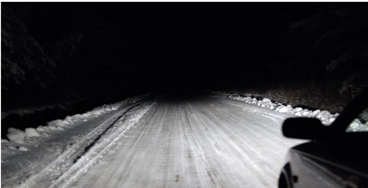
Figure 2-6: Road surface illumination with low beam headlights
