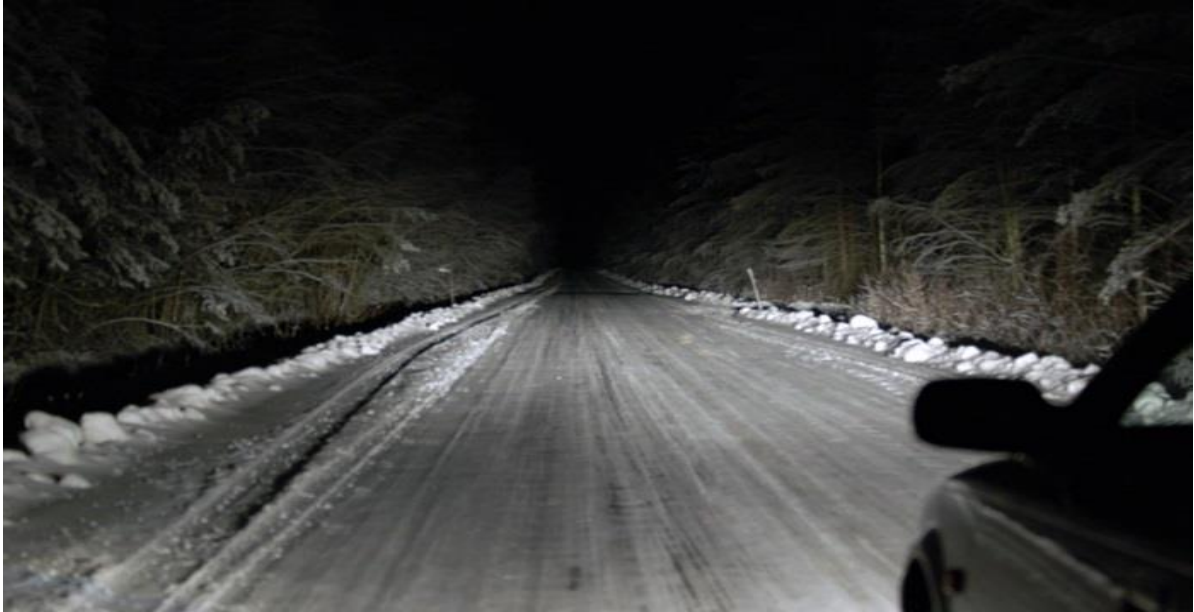
Figure 2-5: Road surface illumination with high beam headlights
