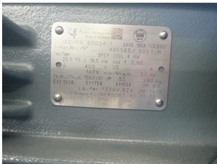
Figure 4-2: SPER 200 L4, 18.5 kW wound rotor induction machine nameplate.
