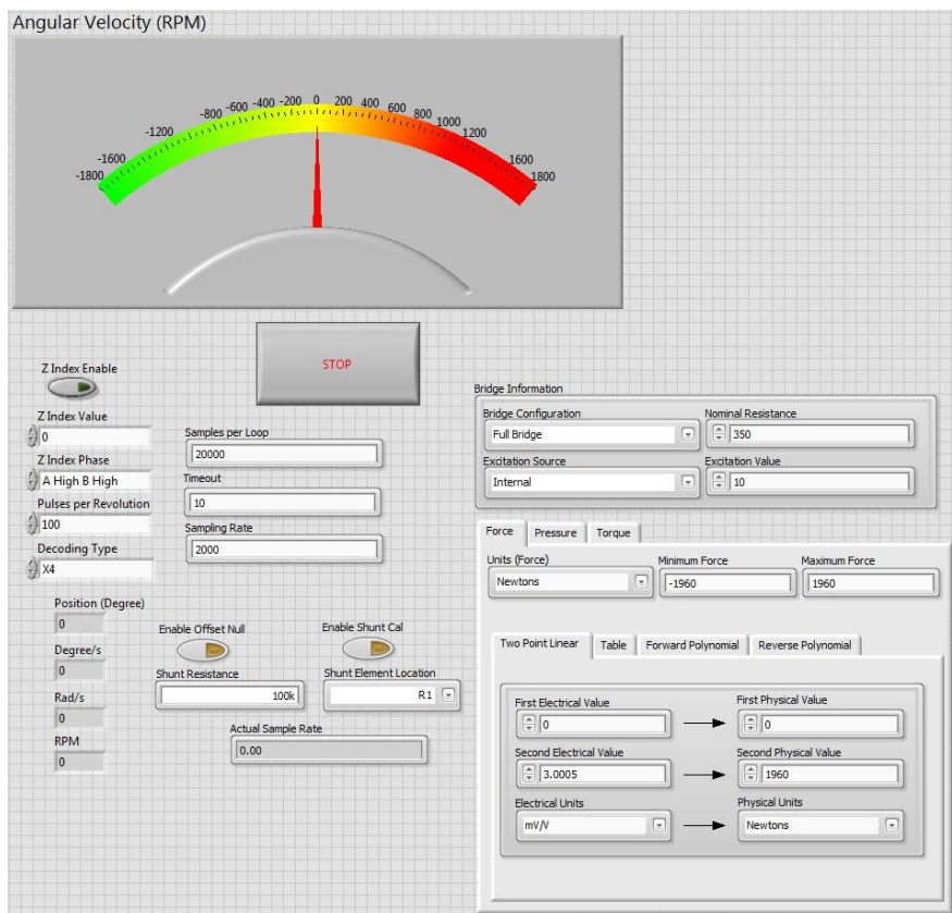
Figure 4-20: Front panel of the codes written for the measurements including the settings in Labview.
