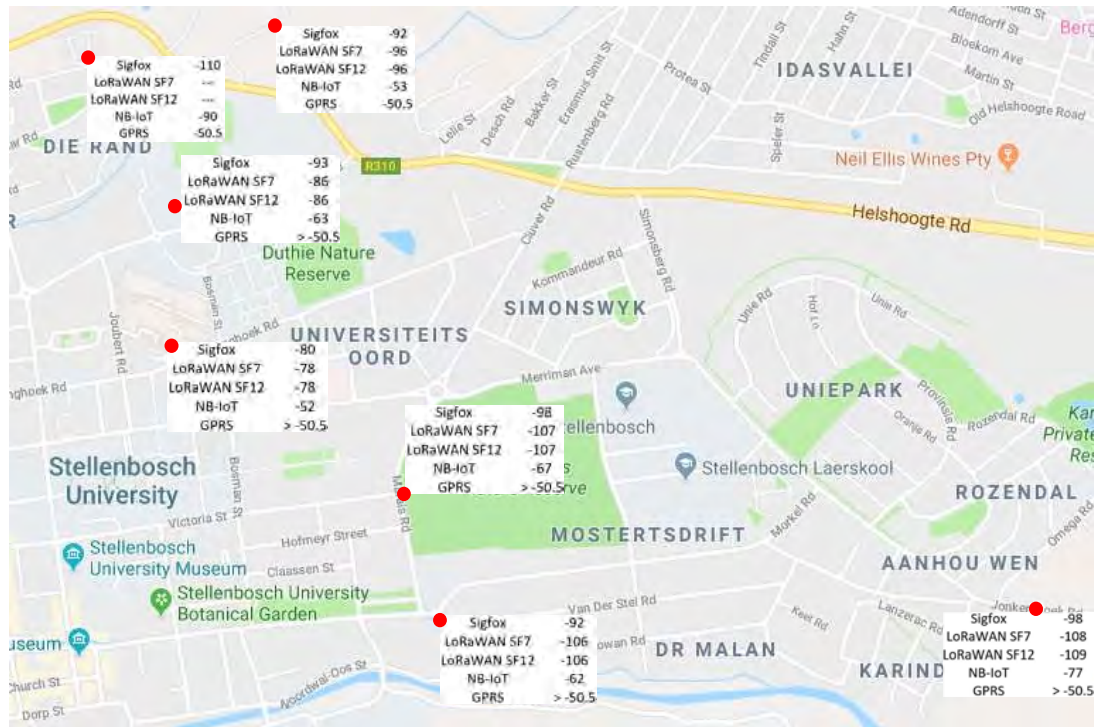
Figure 4.33: Measured RSSI (dB) network coverage of the different networks in the testing area
