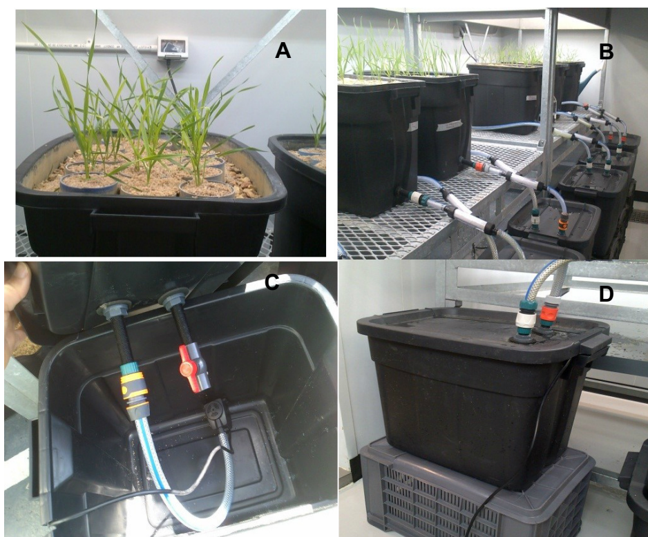
Figure 3.5: Reticulated hydroponic system used. A-ART with plants, B-Complete set of RHS with irrigation system installed, C-Submersible pump for pumping up nutrient solution, D-ART fully-filled with nutrient solution.
