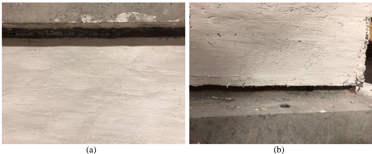
Figure 5.15: SW-100-200-02 2 cm horizontal grooves at (a) top and (b) bottom.
