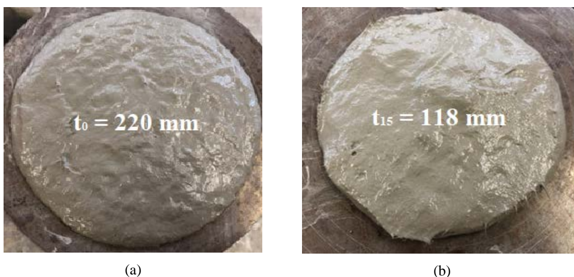
Figure 4.9: Slump flow test (a) directly after mixing, and (b) 15 minutes after mixing.
