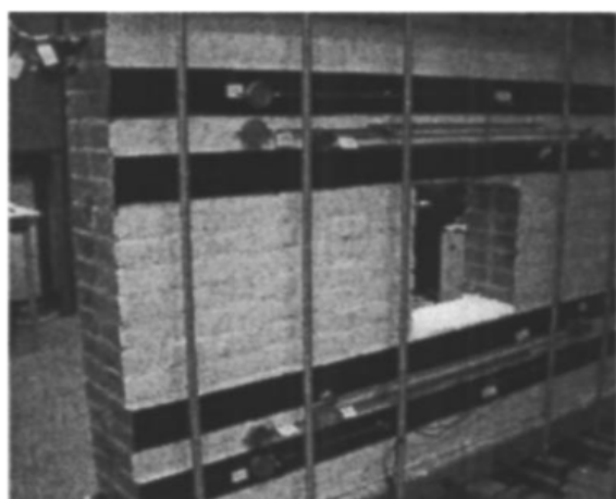
(a) CFRP strips
