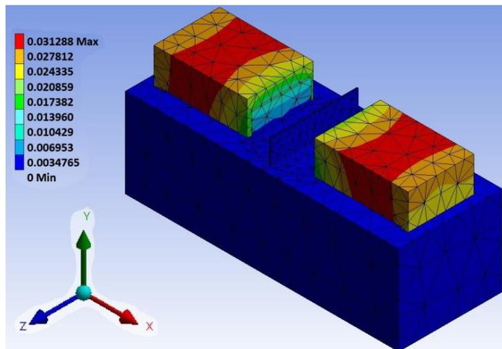
Figure 6. Total deformation of finished part method 2
