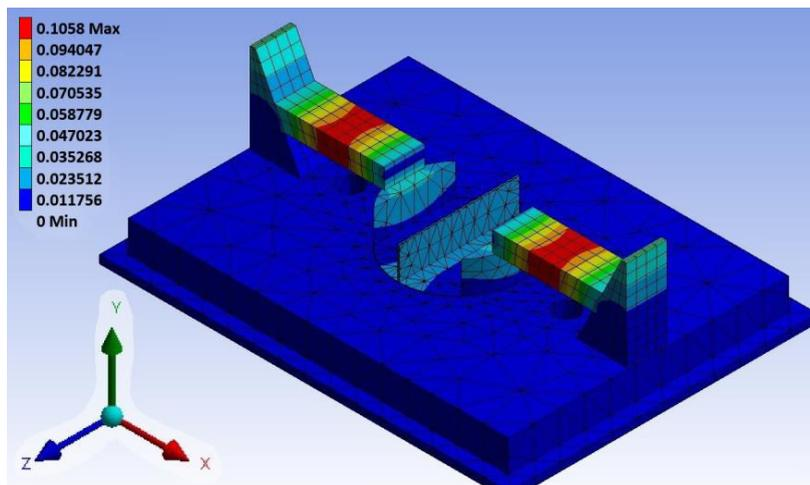
Figure 5. Total deformation for original clamping method
