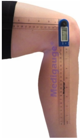
Figure 23: A digital goniometer used to measure the angle between the upper and lower leg (Mediagauge, 2017)
