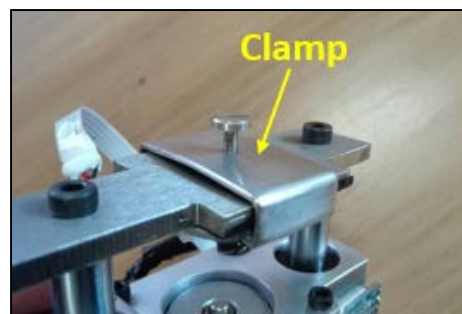
Figure 35: Clamp holding the load cell to the femur plate
