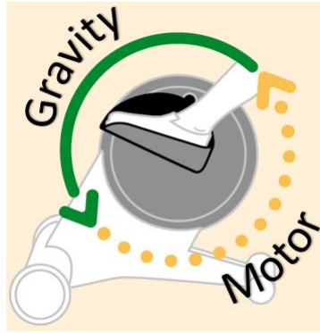
Figure 3.12: Gravitational effect during assisted motion (adjusted from [47])
