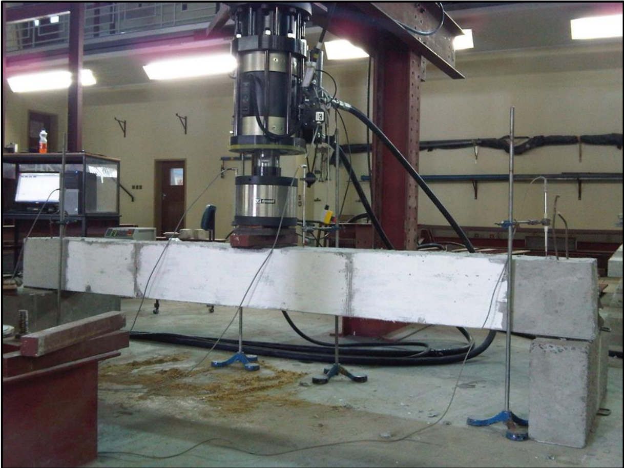
Figure 3-1: Beam testing Setup
