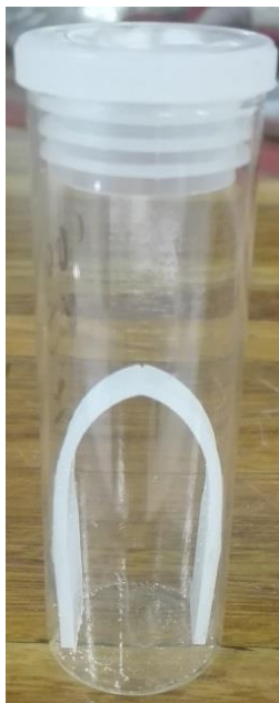
Figure 4.4. Modified bending test setup.
