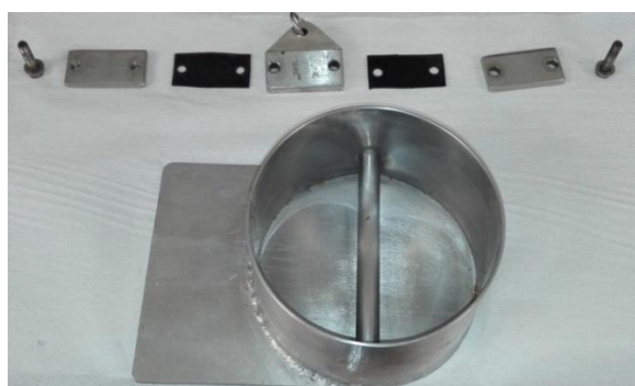
Figure 4.1. Special equipment used for testing ESCR of ethylene based plastics.
