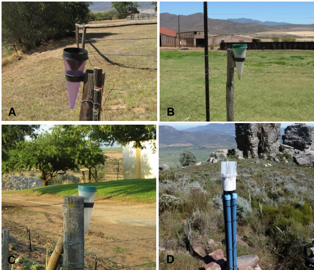
Figure 9: Daily rainfall collectors KA-R2 (a), KK-R (b), VL-R (c) and cumulative rainfall collector M-R (d)
