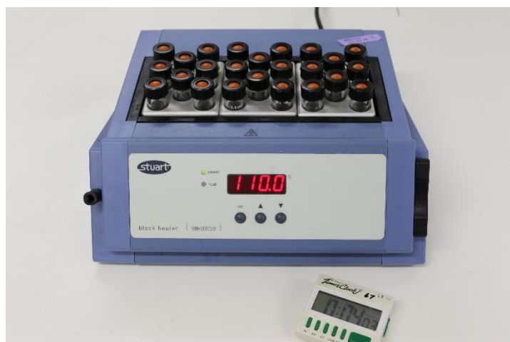
Figure 2 Photo depicting the experimental set-up – Stuart heating block, thermostatted to a specific temperature (110 °C), containing 24 micro reaction vessels.
