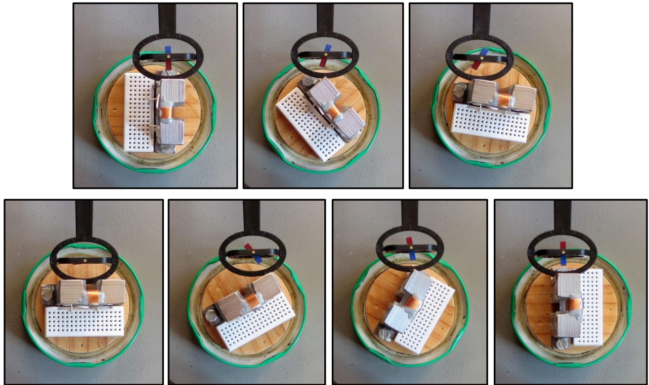
Figure 57: Magnetic field lines indicated by search pole
