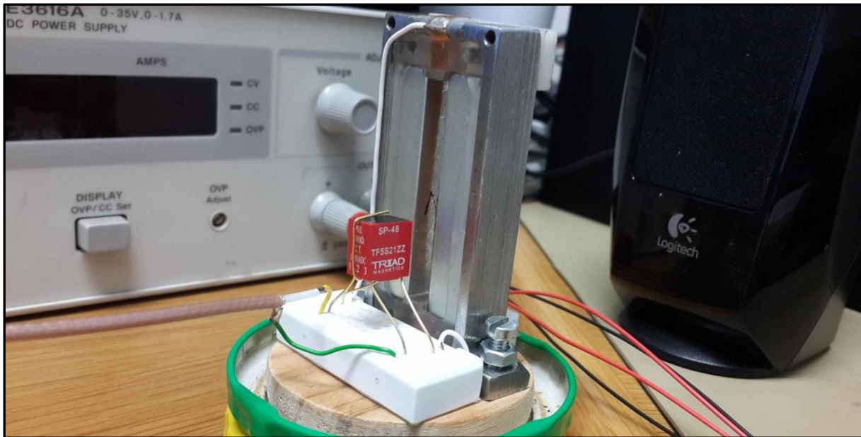
Figure 86: Ribbon microphone and SP-48 transformer
