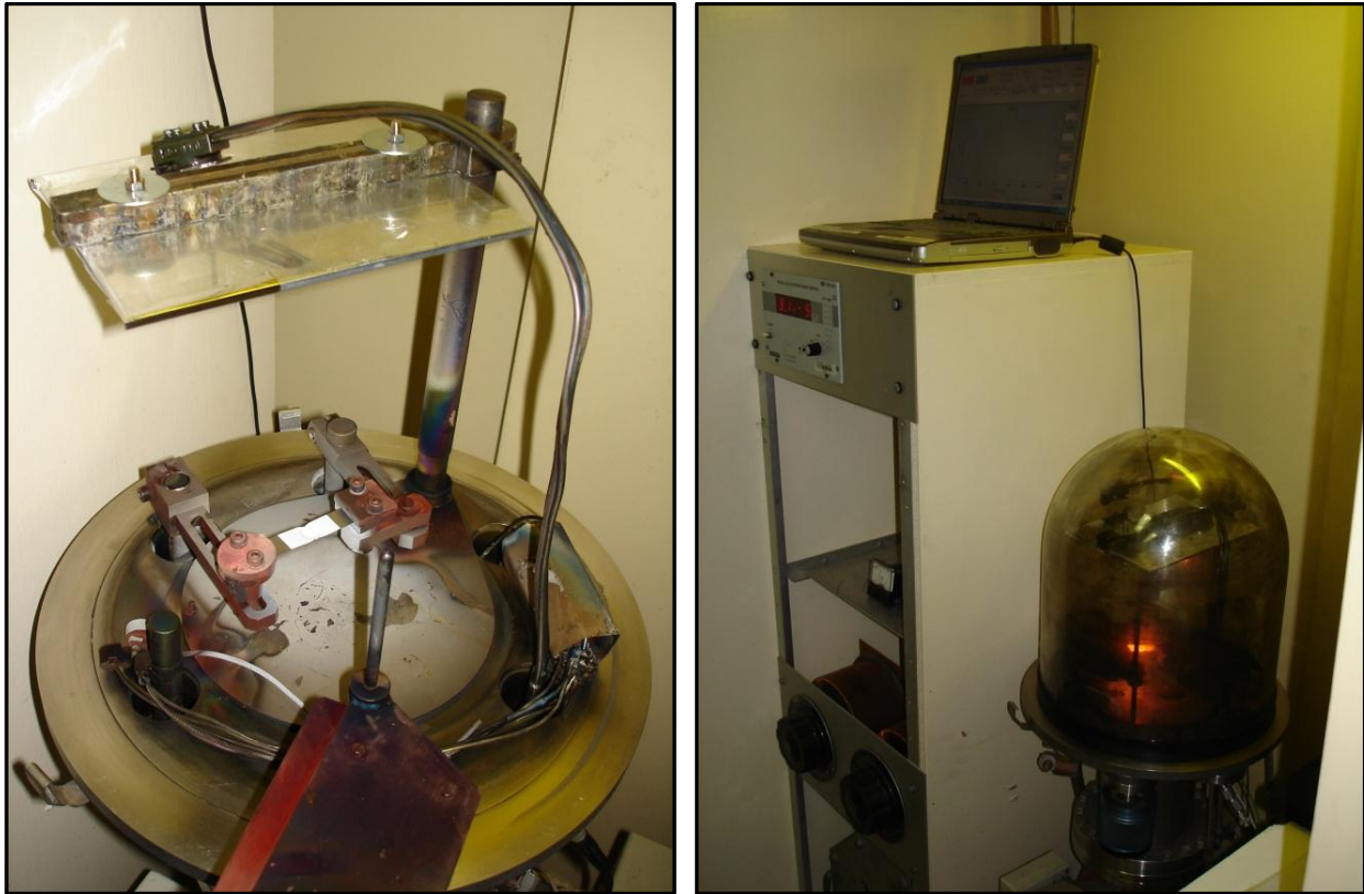
Figure 11: Vapour deposition equipment setup
