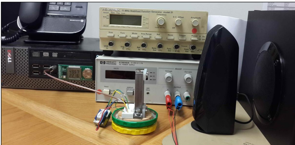
Figure 85: Test setup with ribbon microphone and RMX-1 transformer
