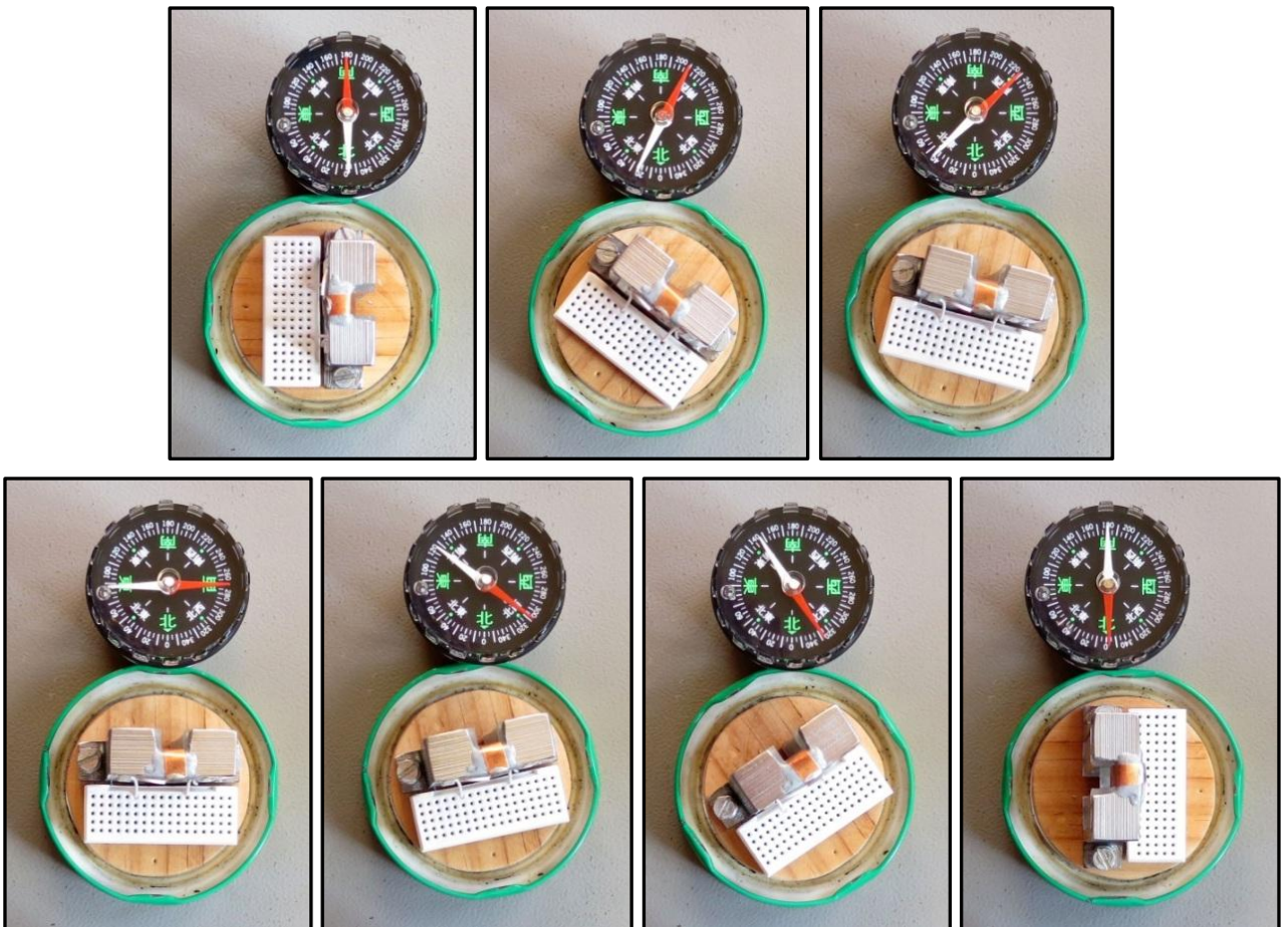
Figure 58: Magnetic field lines indicated by magnetic compass
