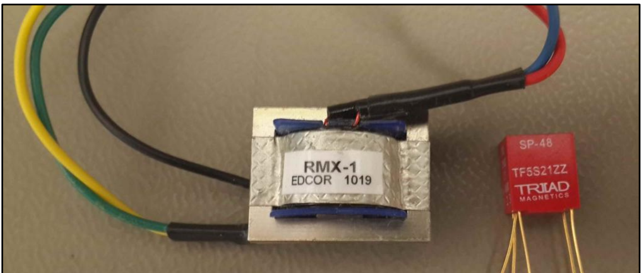
Figure 73: RMX-1 and SP-48 transformers
