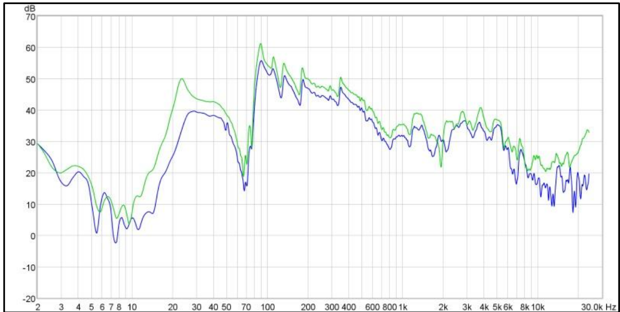
Figure 88: Microphone frequency response with RMX-1 (blue) and AD8321 (green)
