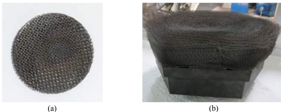
Figure 2.4: Metallic absorbers (a) wire mesh screens (Avila-Marín et al. , 2013), (b) knit wire absorber from the Phoebus-TSA receiver (courtesy of F Dinter at PSA, 2016)
