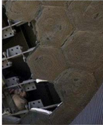
Figure 2.6: Hexagonal cups filled with knit wire in the Phoebus-TSA receiver (from (Avila-Marin, 2011))
