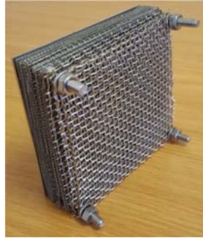
Figure 3.4: Mesh configuration mounted on perforated back plate as absorber
