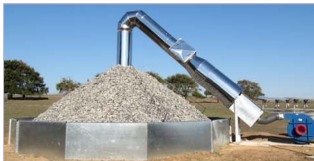
Figure 2.8: Rock bed TES test facility (courtesy of HF Laubscher)
