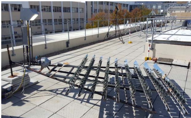
Figure 5.4. Medium flux concentrator with the tower installed for testing
