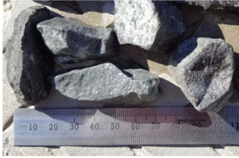
Figure 5.3: Sample of the rocks used in the rock bed heat exchanger
