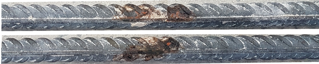
(b) R2 - single crack
