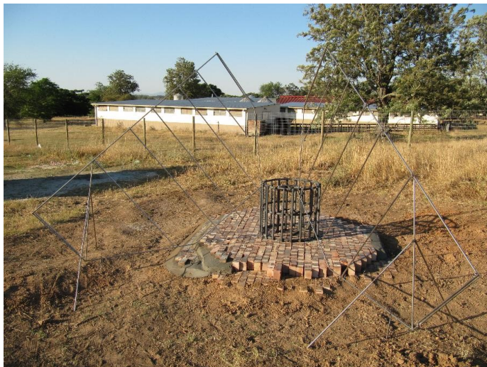
Figure 3.6: Thermocouple placement frame and air distribution box on the thermal energy storage base
