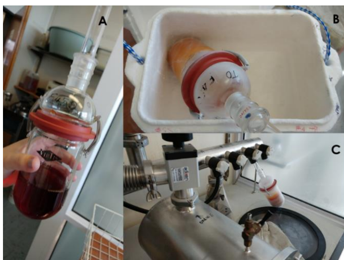
Figure 4: Tea preparation for freeze drying. A) Tea is placed in virtis cryogenic flask. B) Tea is placed in liquid nitrogen for shelling. C) Tea is added to the vacuum for freeze drying.
