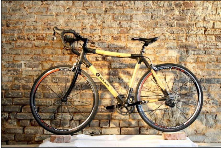
Figure 5.5: Illustration of the bamboo bicycle designed and manufactured by HeroBike
