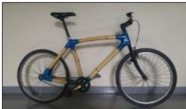
Figure 4.10: Finished bamboo bicycle manufactured at Stellenbosch University
