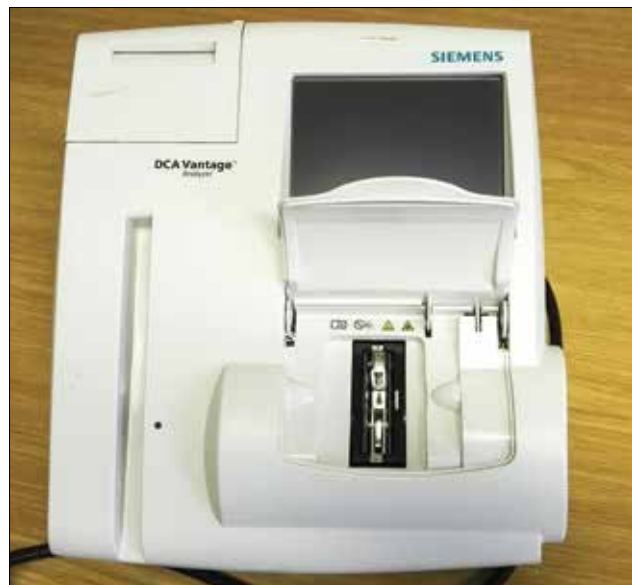
Fig. 1. The DCA Vantage Analyzer for POC testing in a primary care facility.
