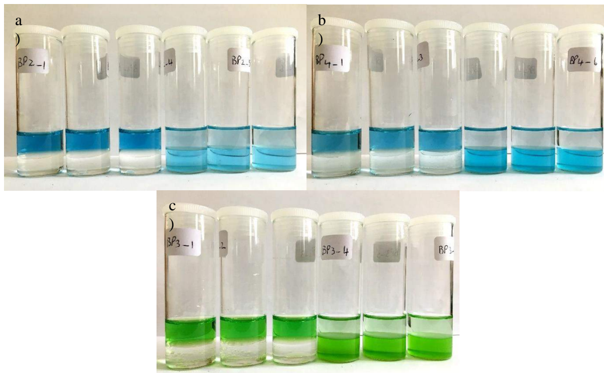
Figure 3.22: Varying colours of the aqueous (top layers) and organic phases (bottom layers) during competitive extraction studies using a) ligand 5 , b) ligand 6 and c) ligand 7/7' . In each picture, the first three polytops (left) represent competitive extractions without the use of synergist, while the following three polytops (right) represent competitive extractions in conjunction with the synergist, SDBS.
