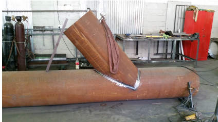
(a) Lateral tee test piece with branch welded to barrel.
