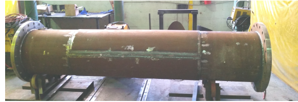
(b) Longitudinal weld on opposite side of branch.
