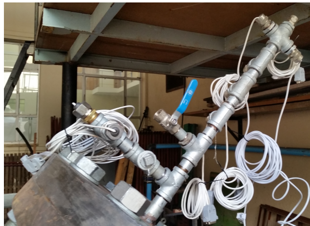
Figure 4.4: Sealing of internal strain gauge cables.
