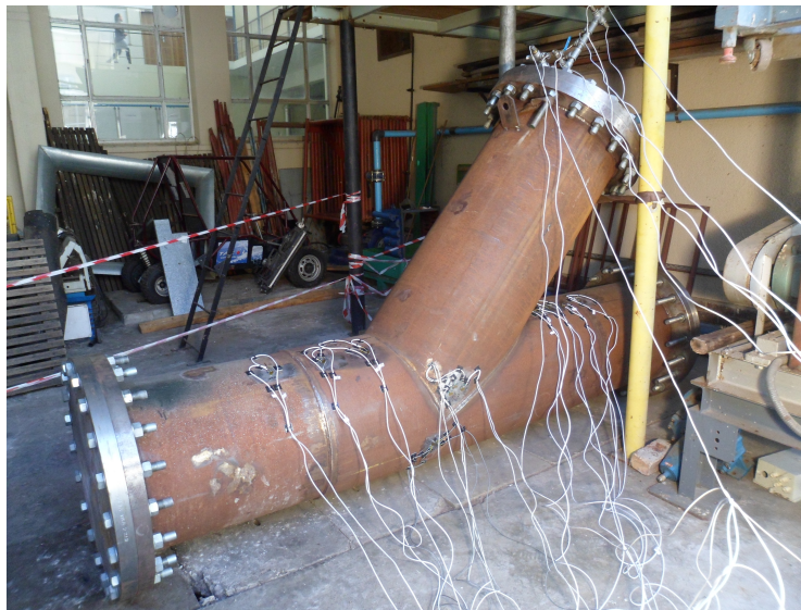
Figure 4.7: Test piece with strain gauges and cables.
