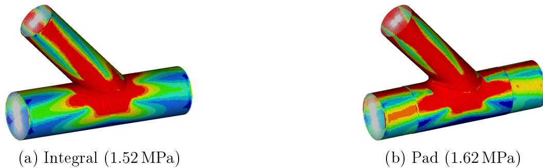
Figure 3.27: Integral vs. pad reinforcing.
