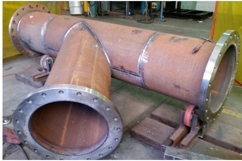
(a) Wrapper halves welded to the barrel.
