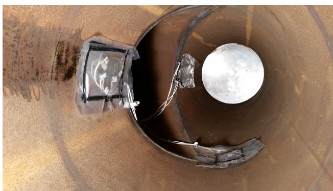
(a) Strain gauges on internal surfaces of special with blank flange on barrel end visible.
