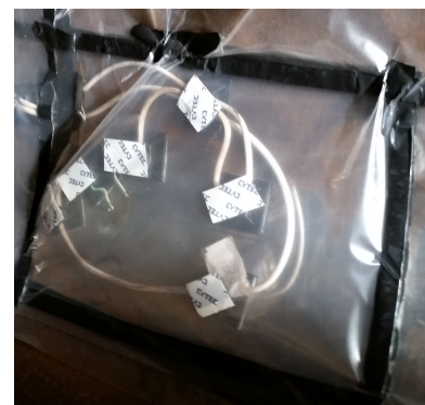
(b) Waterproof sealing over strain gauges.
