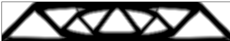
Figure 2.7: Optimal topology generated with convergent SAO of the slope constrained MBB design problem with \mu = 30 and 200 random starts \mathbf{0} \leq \mathbf{t}^{\{k\}} \leq \mathbf{1} : k = 286 , P=600 , f_0(\mathbf{u}^{\{k\}}) = 212.7 , \Theta^{\{k\}} = 5.3\text{D-}5 , d_0^{\{k\}} = 2765 , d_1^{\{k\}} = 2652
