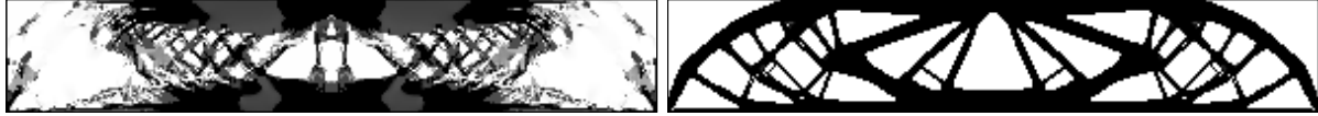
(a) k = 10 , f_0(\mathbf{u}^{\{k\}}) = -3502.6 , \Theta^{\{k\}} = 1.1\text{D}+1 , d_0^{\{k\}} = 1197 , d_1^{\{k\}} = 1875 . (b) k = 54 , f_0(\mathbf{u}^{\{k\}}) = 203.4 , \Theta^{\{k\}} = 9.6\text{D}-7 , d_0^{\{k\}} = 3743 , d_1^{\{k\}} = 3683 .
