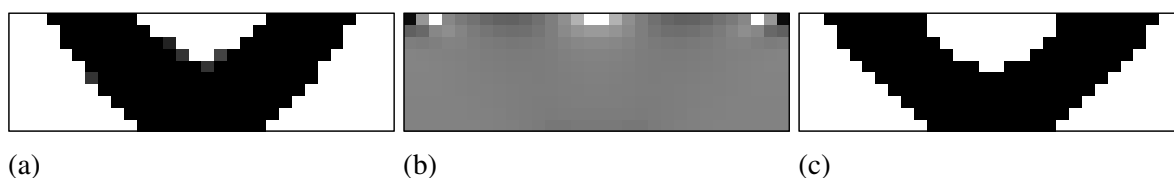
Figure 2.2: Topologies generated for the 2-bar truss design problem; rudimentary SAO with \epsilon = 1 \times 10^{-6} and the (a) nonconvex strategy (b) convex strategy and (c) absolutely nonconvex strategy.
