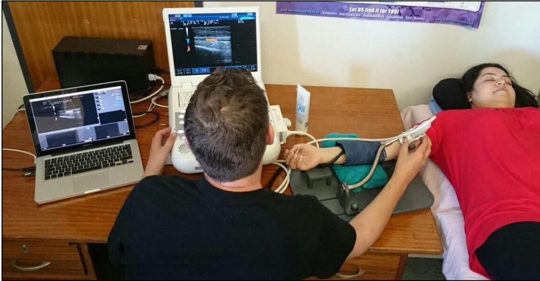
Figure 2.2: A photograph representing a typical FMD assessment with the MyLabTMFive ultrasound and 12 MHz linear probe. On the left, is an Apple Macbook pro laptop with FMD studio and Cardiovascular Suite version 2.8.1. edge detection QUIPU software that records the artery diameter and shear rate throughout the assessment. The study participant is in the supine position with the right arm resting on the probe-holder platform. (This photograph features individuals from the study research team, and consent was given by both individuals to include it in the thesis).
