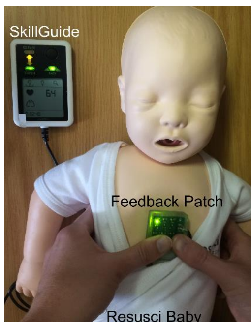
Figure 3.8: Feedback test showing the green LED, indicating correct depth.
