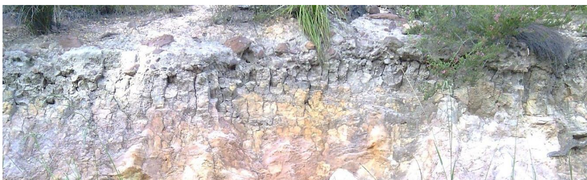
Figure: 6.5 Shallow topsoil above prismatic structure on top of saprolite.
