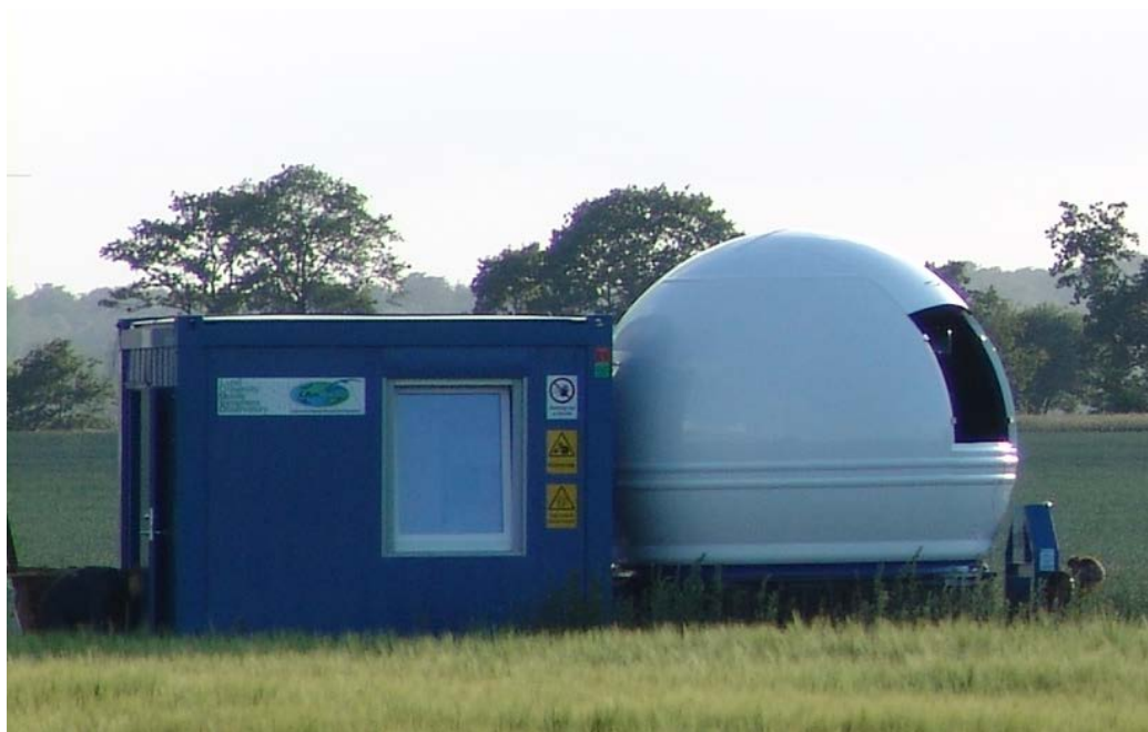
Figure 22: LUMBO: It has two main parts the blue container in the left is a control room. The white dome is where the five telescopes and detectors are placed. The dome is motorized and can rotate 360°. The field of view opens 90°
