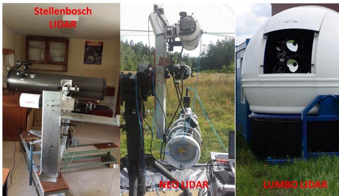
Figure 33: Scheimpflug LIDAR Setup: Left: Stellenbosch kHz remote sensing setup. This works both in active and passive mode using laser and sunlight as illumination source respectively. Middle: Norway electro-optics (NEO) continues wave laser radar setup. This was designed for the active mode using 808nm IR laser light source. Right: Lund university mobile biosphere observatory (LUMBO) setup, which is multipurpose mobile system capable of insect monitoring and bird tracking.
