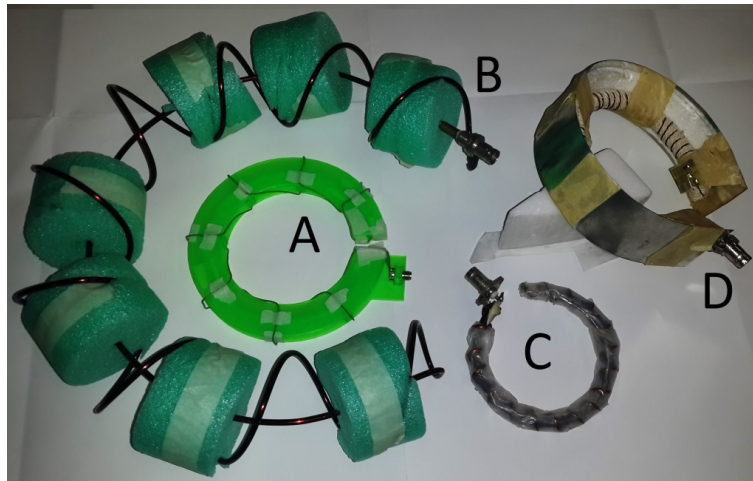
Figure 2.5: Some of the Rogowski Coils used in this project. A: a low profile RC, B: the large RC which was the main focus of this study, C: a smaller RC, D: an RC with an electrostatic shield and terminating resistance.
