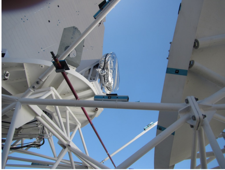
Figure 4.13: Safety measures to ensure that the L-band receiver is not damaged.
