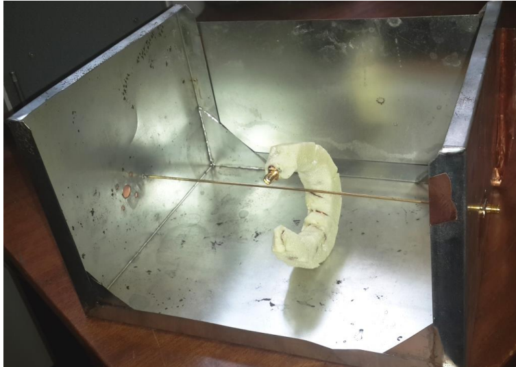
Figure 3.16: Small fixture (250 mm in length) used in the high permittivity experiment. Only one of the added walls is present. A newly fabricated RC was made with polyurethane foam to keep the permittivity of the dielectric between the windings close to 1.
