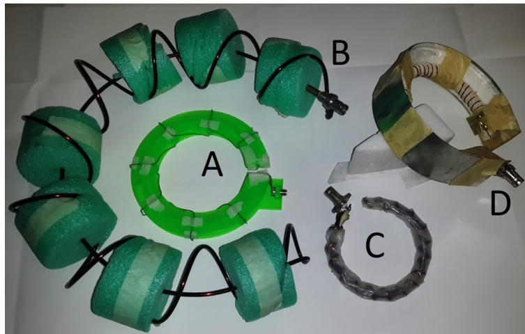
Figure C.1: A set of different Rogowski coils. A: a low profile RC, B: the large RC, C: a smaller RC, D: an RC with an electrostatic shield and terminating resistance.
