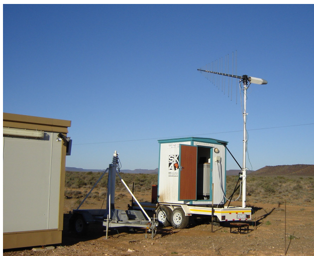
Figure 4.3: The RFI trailer used in some of the captures. Photo credit: Paul Manners (SA-SKA/HartRAO).
