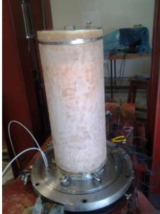
Figure 3- 27: Large-scale Tri-axial Specimen Placed on Baseplate
