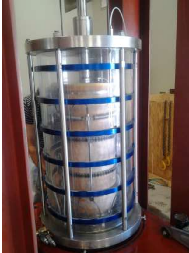
Figure 3- 32: Large-size Tri-axial Cell Lowered into Position using Vertical Actuator
