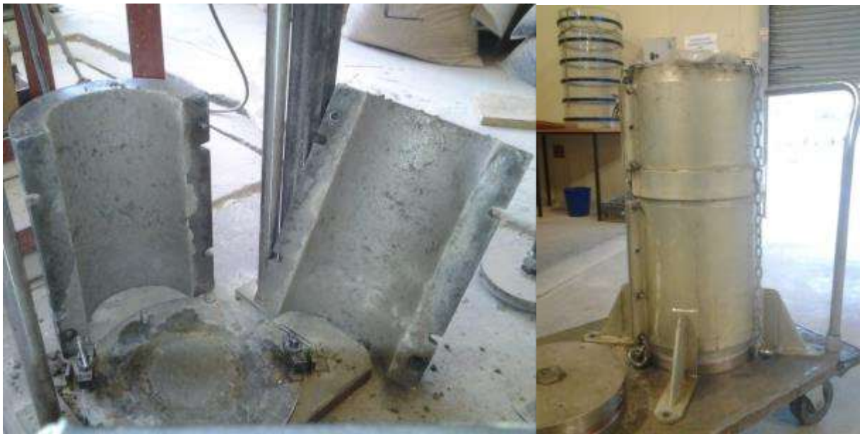
Figure 3- 16: (a) Small-scale Split Mould and (b) Large-scale Split Mould
