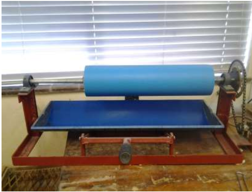
Figure 3- 23: Equipment used for the Manufacturing of small Latex Membranes
