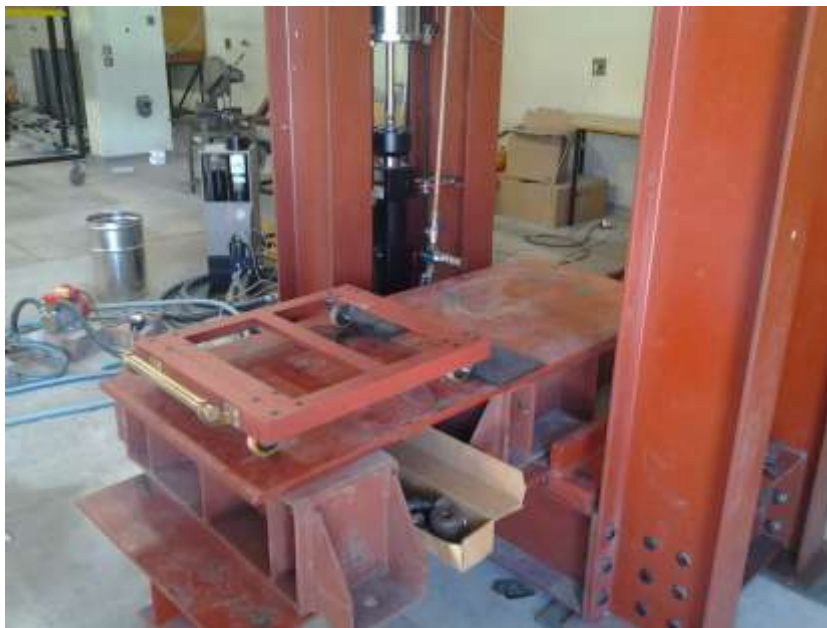
Figure 3- 29: Trolley Designed and Built to Assist Moving of Tri-axial Cell
