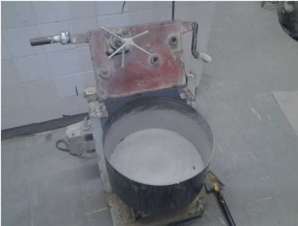
Figure 3- 14: Pan Mixer used to Mix Material
