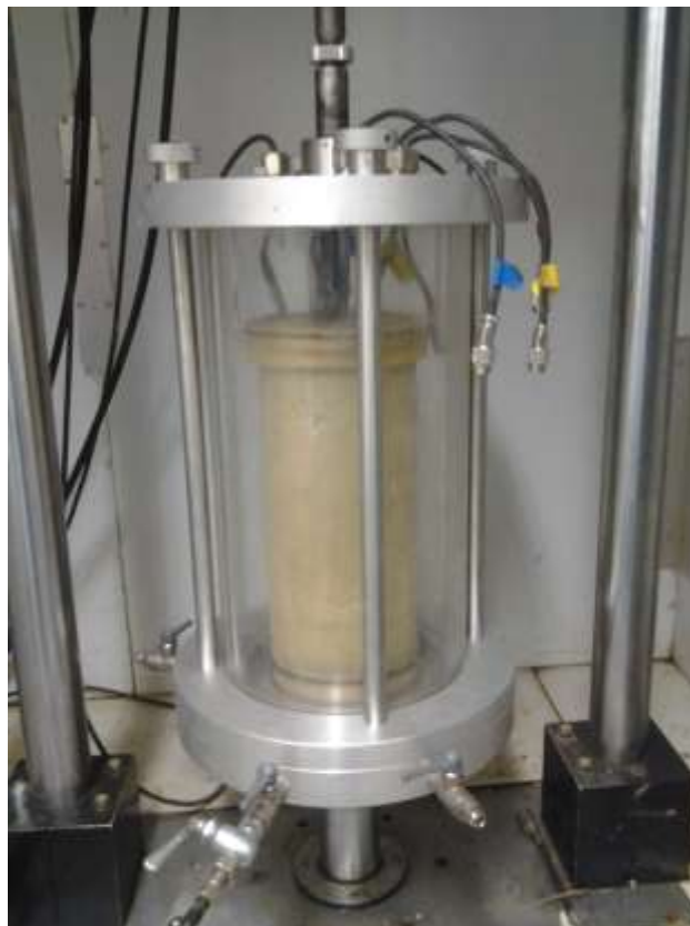
Figure 3- 25: Small-scale Tri-axial Specimen Assembled for Monotonic Testing
