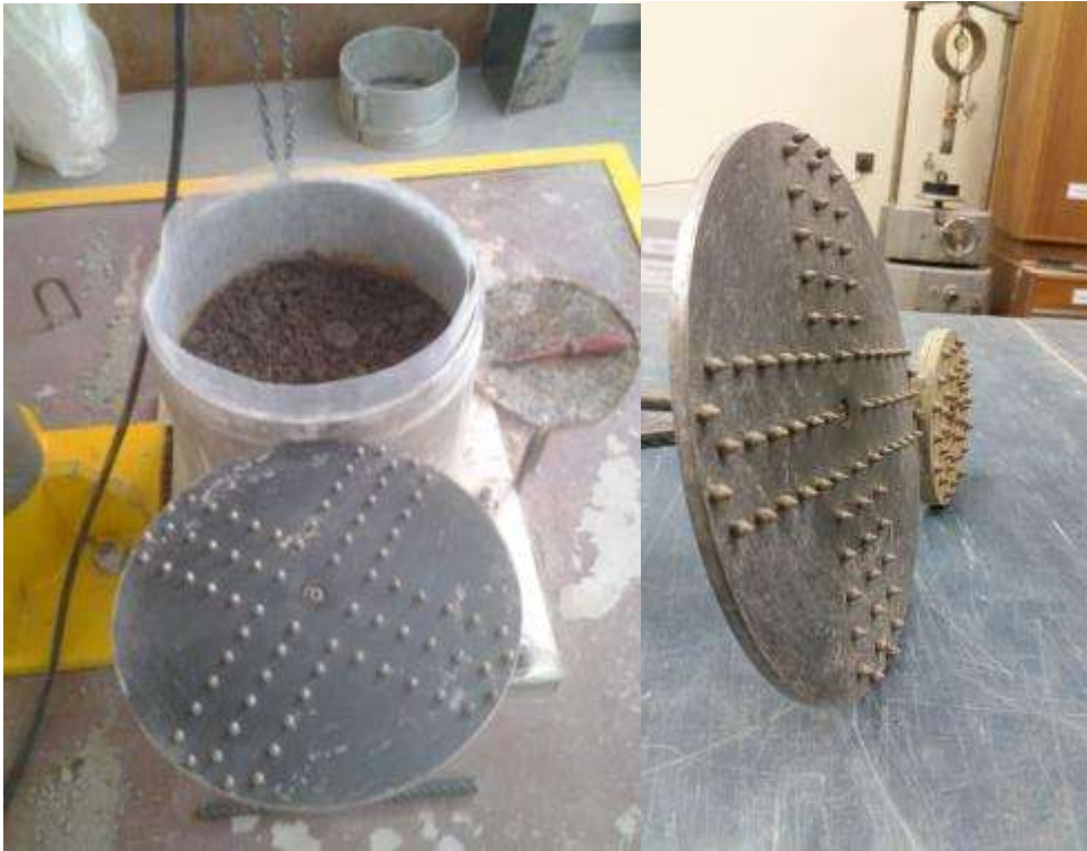
Figure 3- 19: Scarifying Tools used to Loosen Top of Compacted Layers
