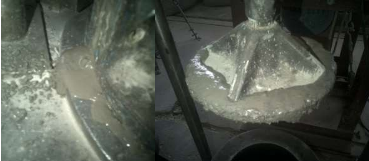
Figure 3- 9: Material Slush Forced from Mould at Excessively High Moisture Contents
