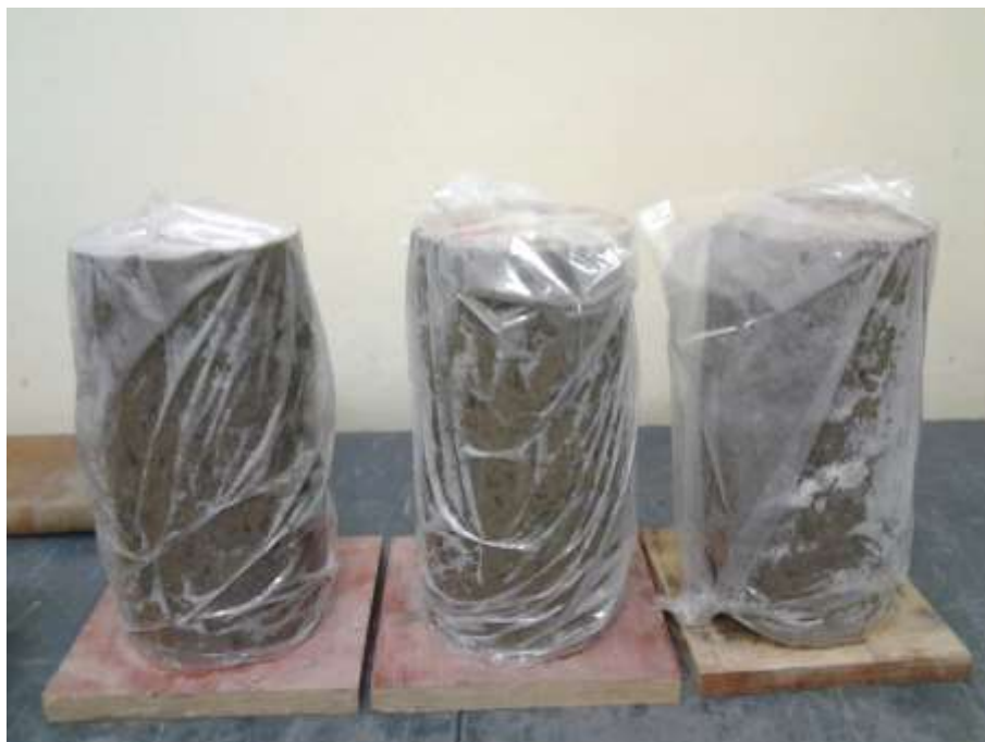
Figure 4- 3: Moisture Adhering to Plastic Surface during Curing
