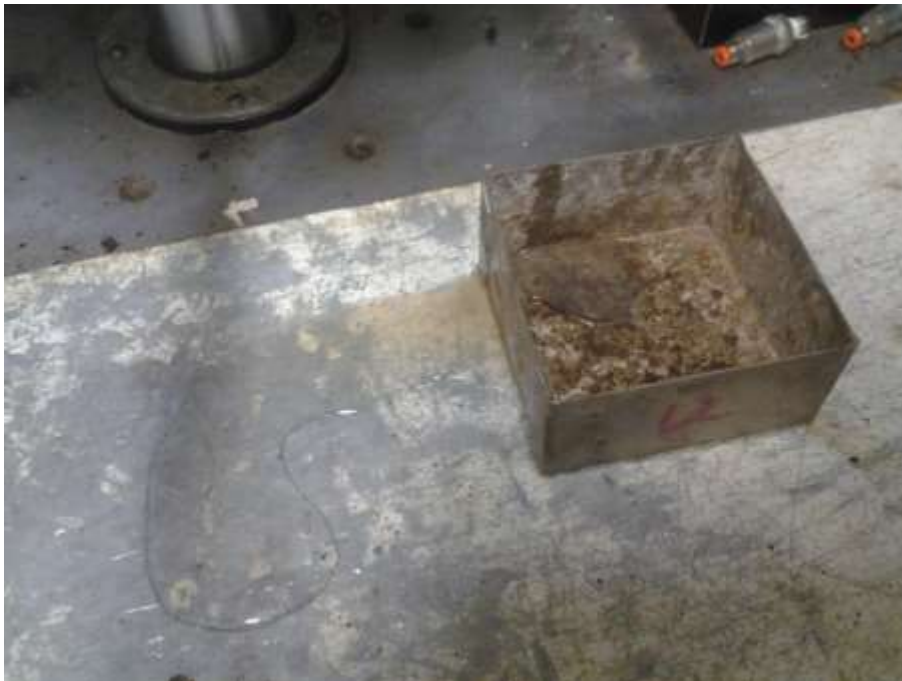
Figure 4- 4: Moisture Extruded from Specimen during Dynamic Loading
