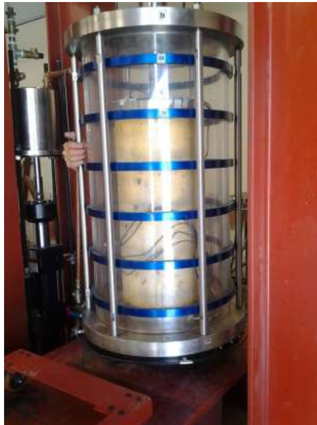
Figure 3- 31: Large-size Tri-axial Cell being Lifted by the Actuator
