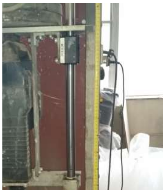
Figure 3- 15: Tape Measure Placed on Vibratory Hammer to Control Layer Thickness/Density
