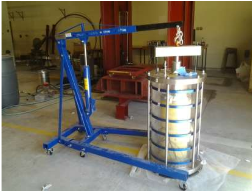
Figure 3- 28: Large-size Tri-axial Cell Connected to Portable Crane
