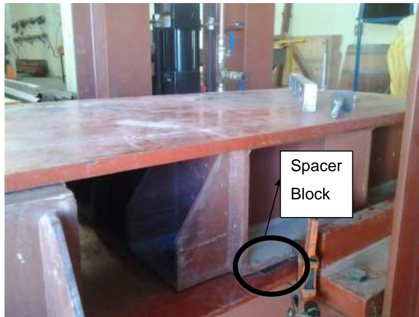
Figure 3- 37: Spacer Blocks used to Level Tri-axial Platform
