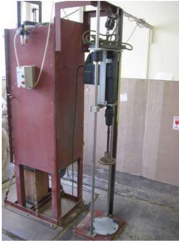
Figure 3- 7: Small-scale Vibratory Hammer Setup with Bosch Hammer
