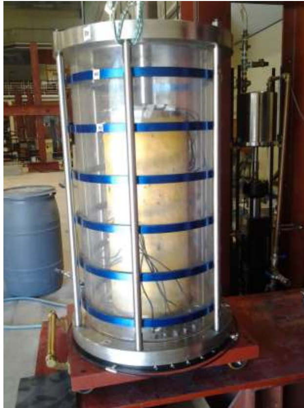
Figure 3- 30: Large-size Tri-axial Cell On Top of Trolley
