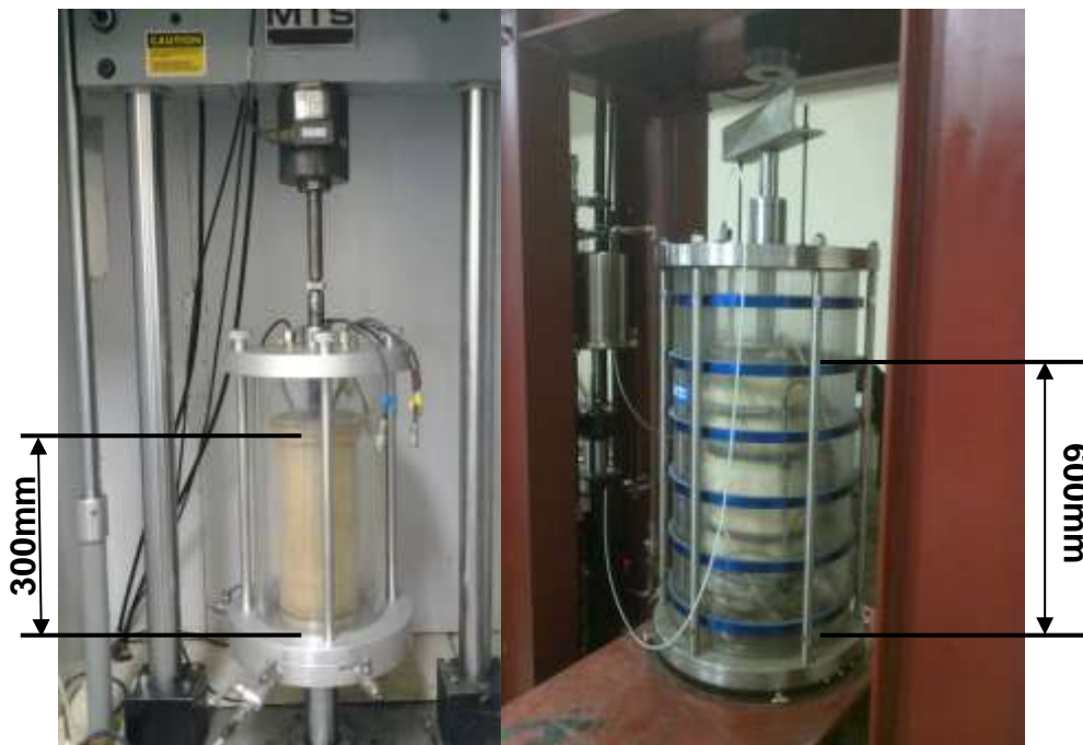
Figure 3- 22: Small-scale (Left) and Large-scale (Right) Tri-axial Testing Device
