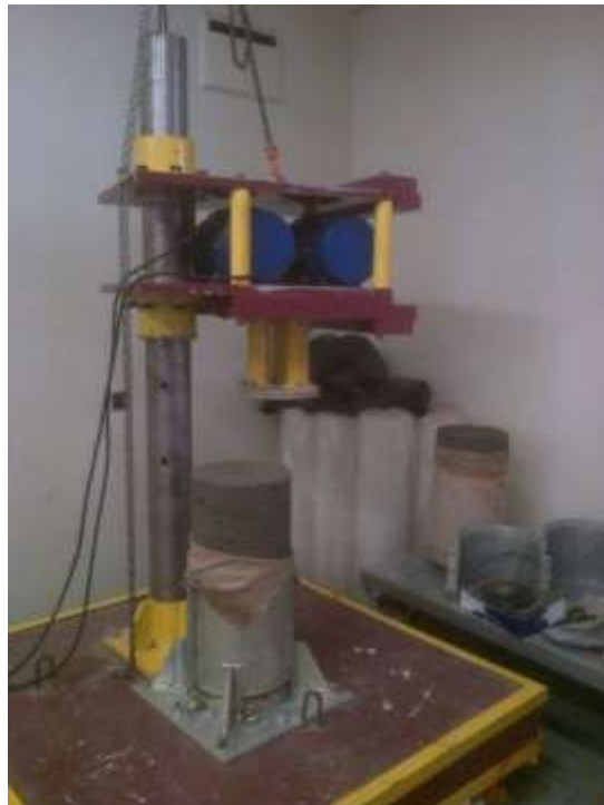
Figure 3- 11: Large-scale Vibratory Hammer
