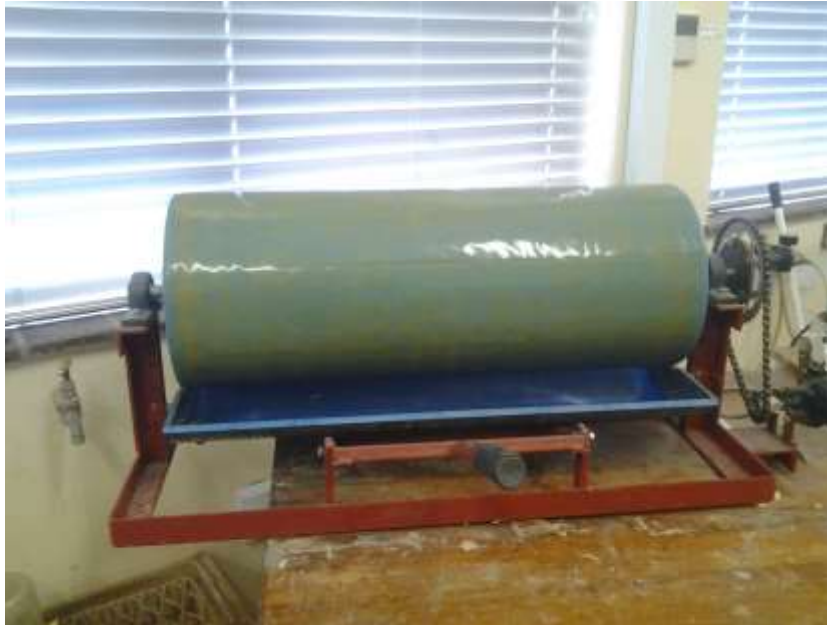
Figure 3- 24: First Layer of Large-size Membrane after Drying
