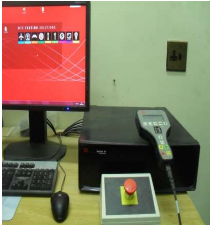
Figure 3- 21: MTS Flextest 40 Controller used for both Small- and Large-size Testing
