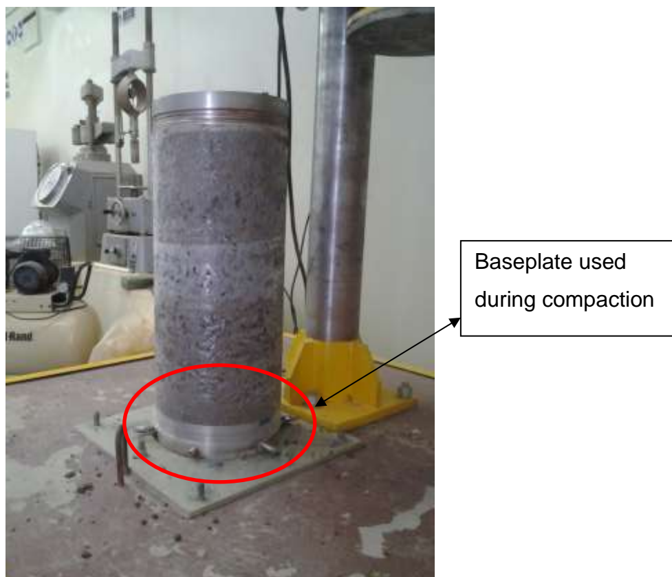
Figure 3- 26: Large-size Tri-axial Specimen Compacted On Top of Baseplate
