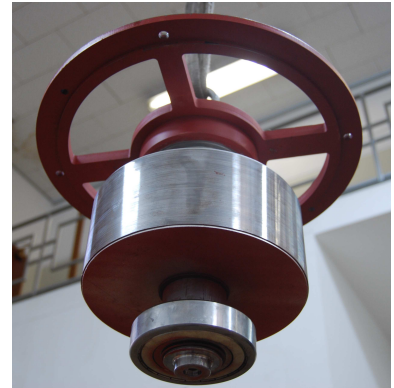
(b) Rotor of the winch RSM lifted into the stator with a crane.
