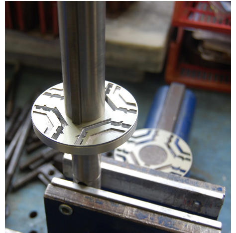
(b) Laminations being stacked on the end-cap.
