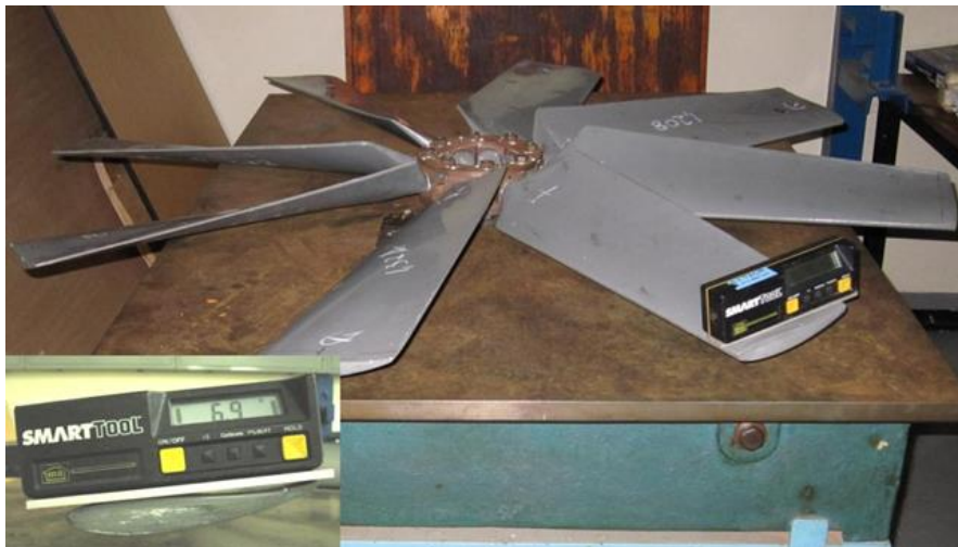
Figure 4.3 - Measuring the blade-setting angle
