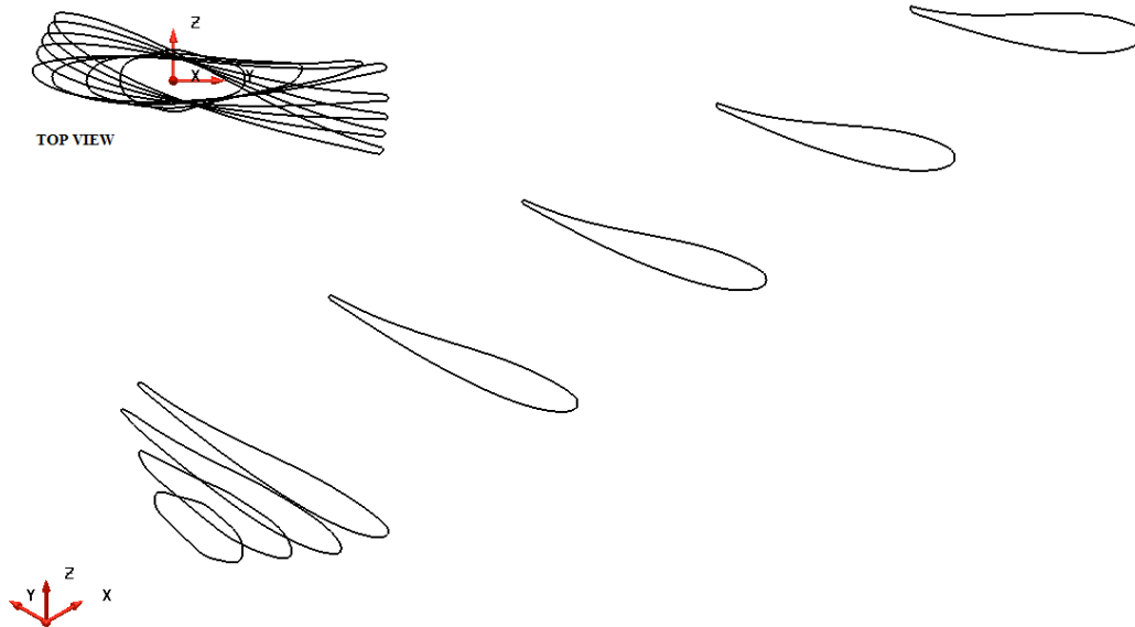
Figure 3.4 - 3D wireframes of the L1-fan scanned by the contact scanner
