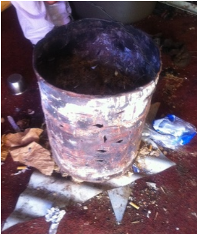
Figure 5.8.1: Wood-fired indoor heater - Enkanini
