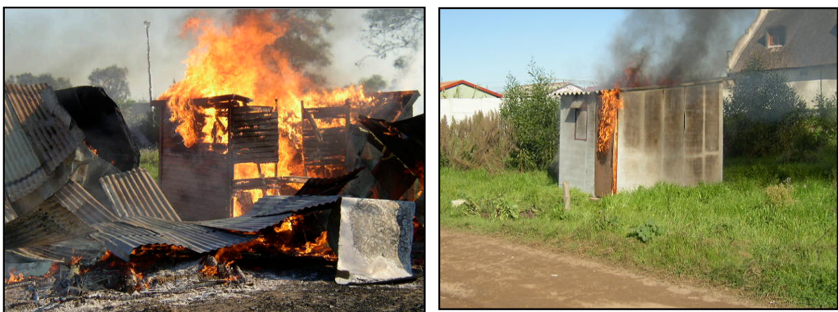
Figure 3.4: Conventional shack after burning for 8 minutes (left) versus Fibre Concrete structure after burning for 47 minutes (right)
