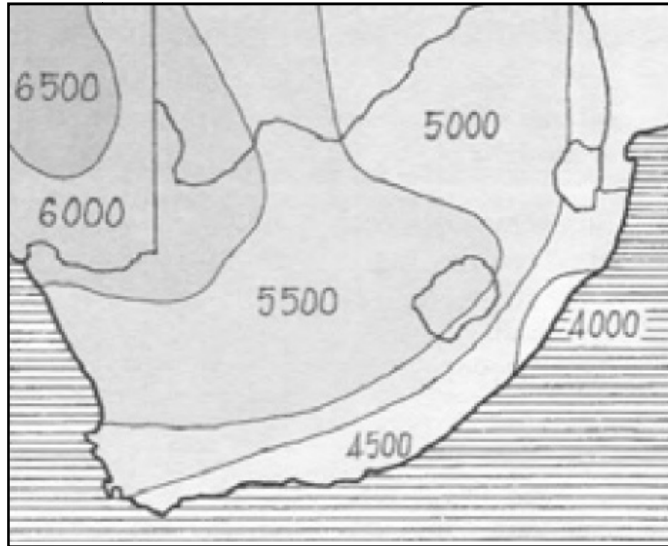
Figure 3.4: Annual solar potential in South Africa in average watt hours per square meter per day (Source: PDG 2007:51)
