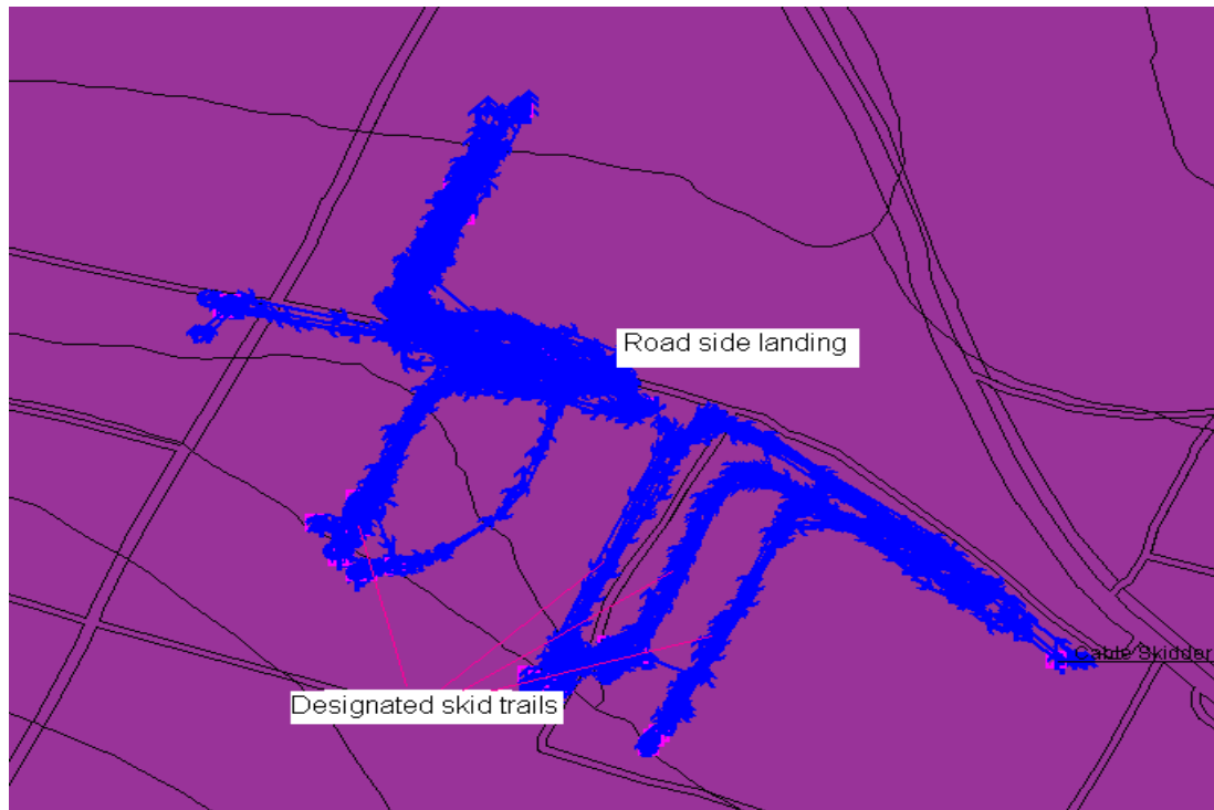
Figure 23: An extract from GPS tracking data showing travel pattern of the skidder in the planning blocks.
