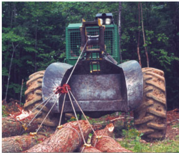
Figure 2: Mainline rigging (source: Wallingford's Inc. http://www.wallingfords.com/wallingfords/winchline_hooks.html ).
