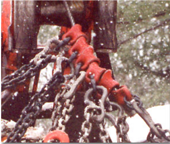
Figure 3: Tagline rigging components (source: Wallingford's Inc. http://www.wallingfords.com/wallingfords/wincline_hooks.html ).
