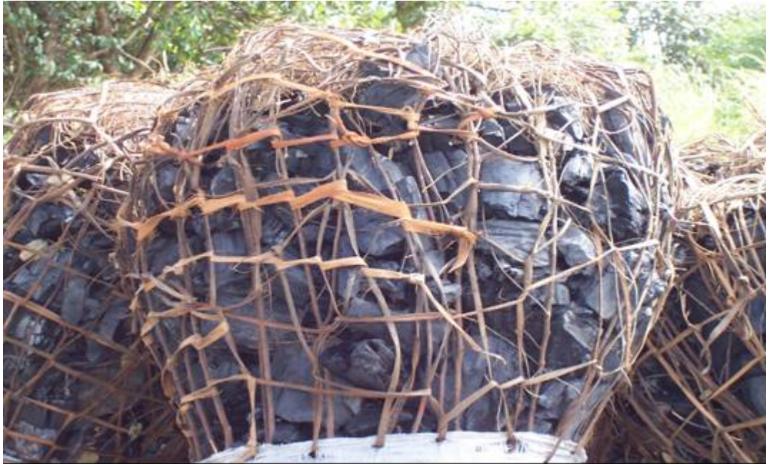
Figure 2.2 Bark rope on the charcoal bag head
