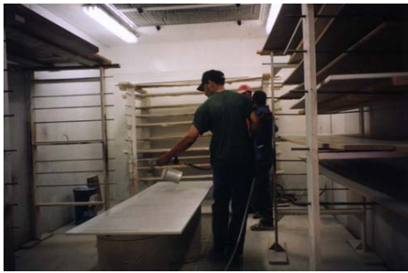
(a) Components sprayed by the spray-painter.
