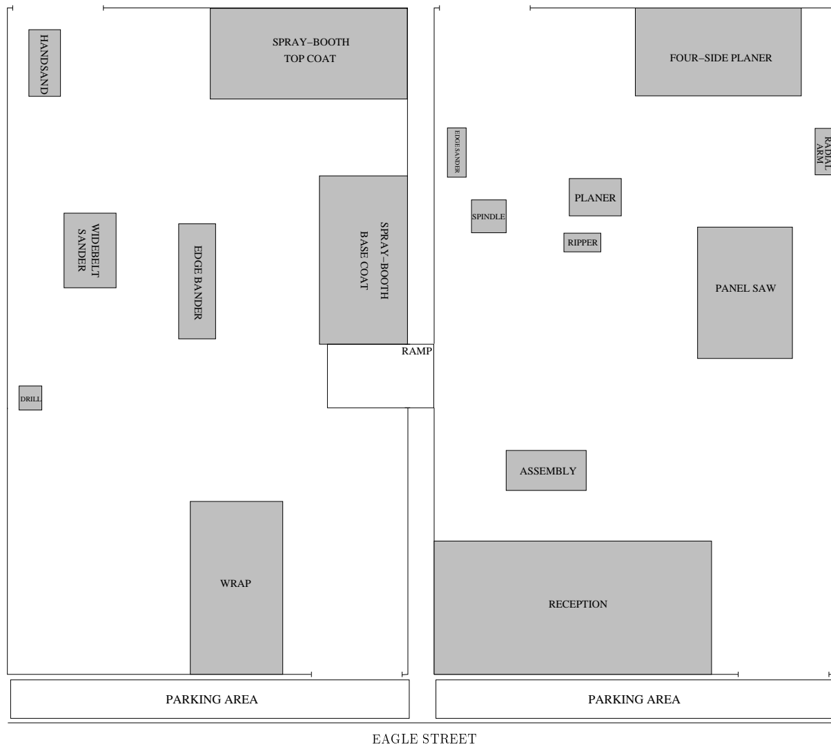
Figure 4.7: The layout of the machines on the LWC factory floor.
