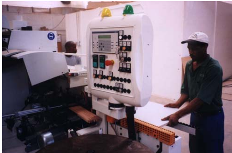
Figure 4.13: Solid wooden edges are inserted into the Edge Bander before a worker guides the component through the Edge Bander.
