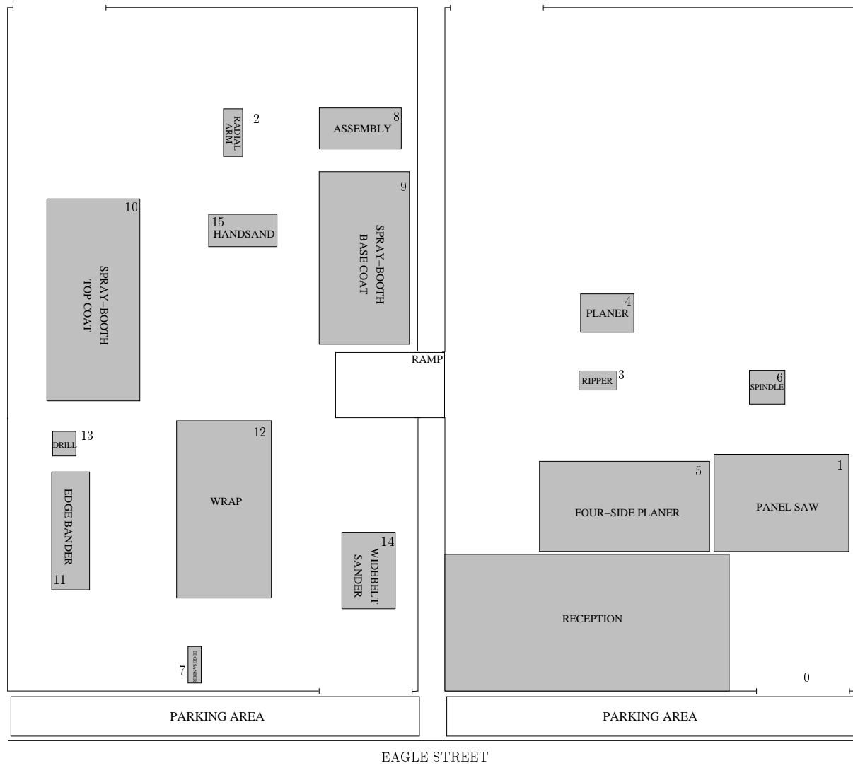
Figure 5.20: Layout obtained after manual changes were made by the LWC management of the layout in Figure 5.19. The large gap at the top of the right hand side of the factory can be used to store all the raw material.
