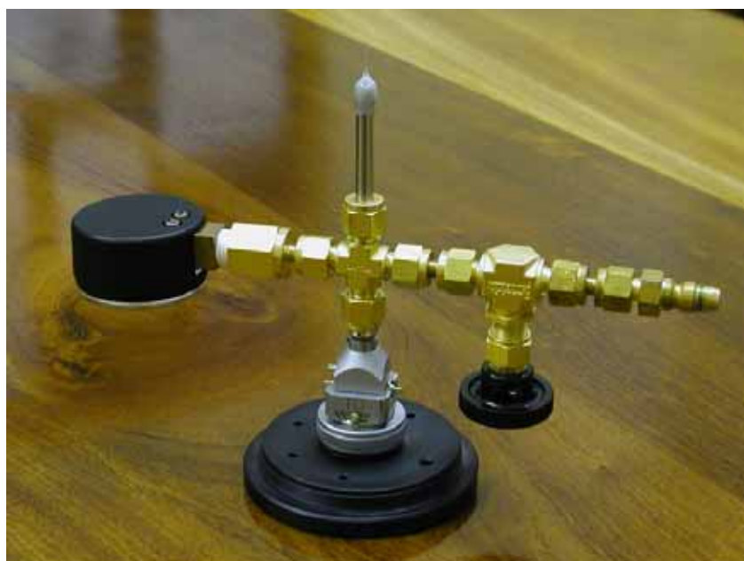
Figure 53. Apparatus used for the determination of crystal structures under mild gas pressures.
