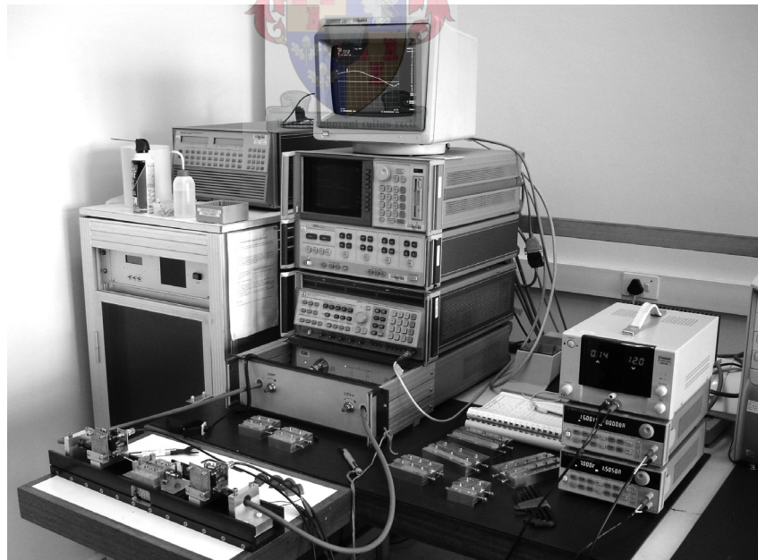
Figure 3.3: A typical automated test setup using a HP8510C VNA to perform the characterisation. The HP6612C power supplies in the right hand side of the figure are used for sweeping the gate and drain voltages using a PC.
