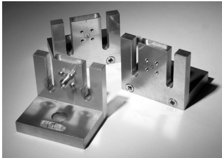
Figure 2.15: Aluminium mounting pieces that incorporate the coaxial to microstrip transitions. The connector tab sticks out so that it can be pressed onto a microstrip calibration standard.
