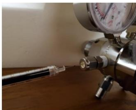
Figure 7. Aspirating a volume of C 2 H 4 through a septum from a pressure regulator
