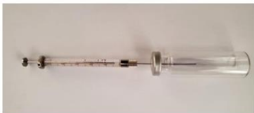
Figure 8. Use of a 100 µL syringe to dilute C 2 H 4 gas in a headspace vial
