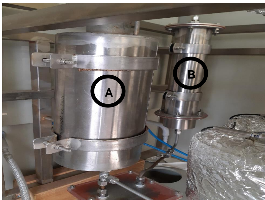
Figure A.4: (a) Regeneration columns and control box; and (b) the condenser A and activated carbon trap B
