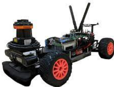
Figure 3.1: An F1/10 th vehicle equipped with hardware for autonomous navigation.
